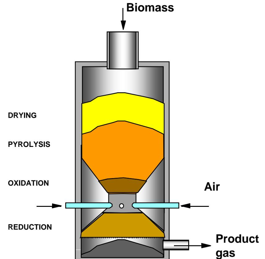
**SME companies are developing small-scale gasifiers for gas engines in Finland aiming to 100 – 500 kWe (at least 5 different companies)**
