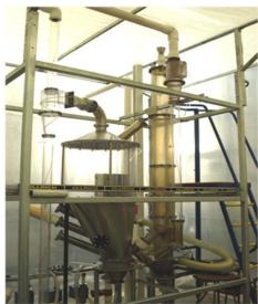
Fig. 8. Cold and transparent DFB model in UoC
