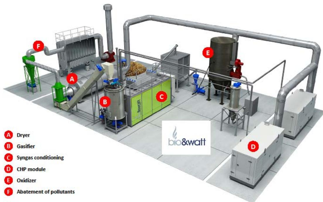
Figure 1: Plant layout and main subsystems
