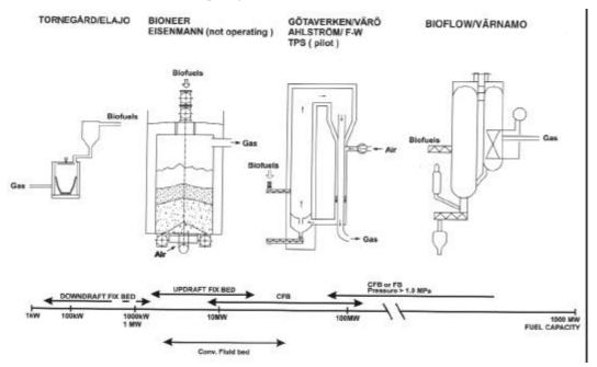
Figure 5 Commercial biomass gasifiers in Sweden
