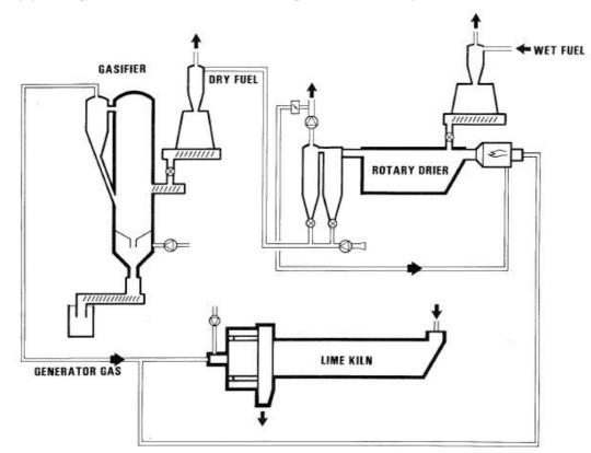
Figure 7 Biomass gasification plant at Värö Mill
