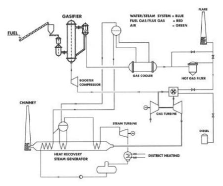
Figure 10 Process diagram of Värnamo plant
