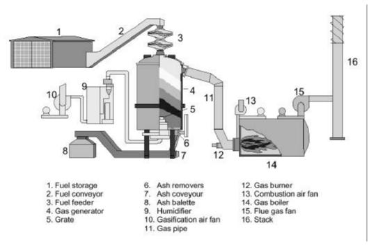
Figure 6 Bioneer updraft gasifier
