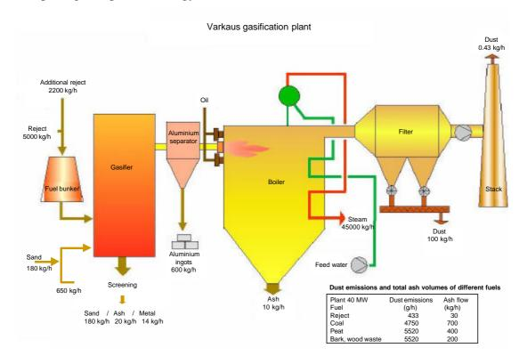
In Corenso's new gasification plant, the fibre material in multi-layer packages is recycled in coreboard, the aluminium being recycled as raw material for foil. The remaining plastic is gasified to create energy. The metal and packaging bands in the loads of collected raw material are sent to the metal industry for recycling. Thus, everything is recovered.
