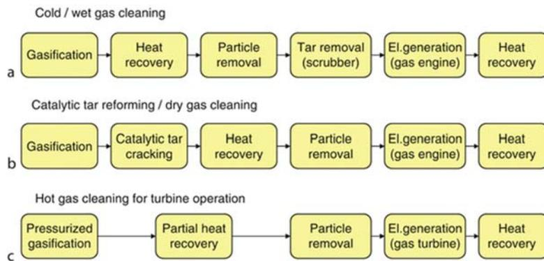
Figure 7: Typical process chain of gas cleaning for CHP applications
