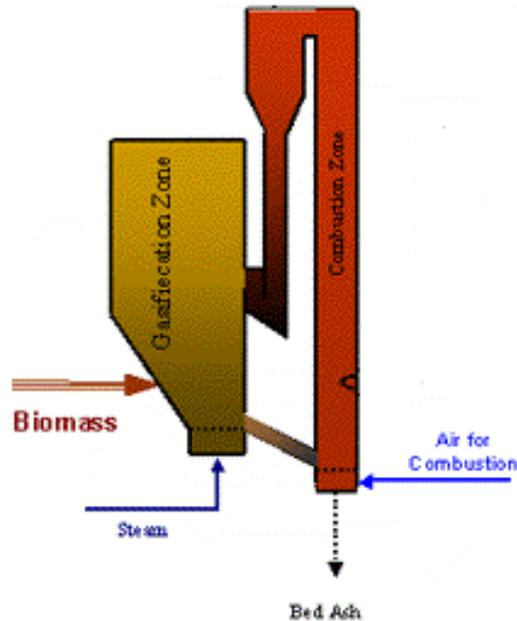
Figure 5: Circulating fluidized two-bed gasifier
