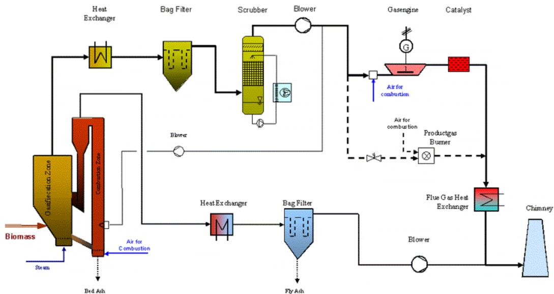
Figure 9: FICB Güssing – flow sheet
