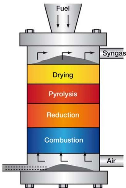
Figure 3: Fixed bed updraft gasifier [1]
