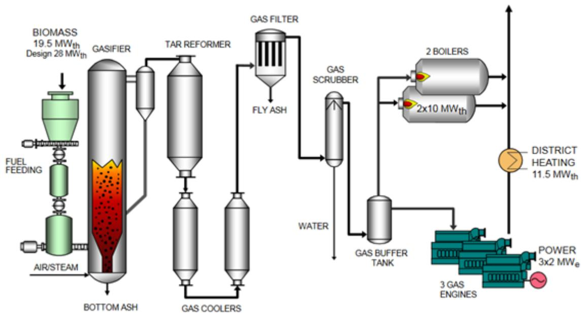
Figure 14: Skive plant – flow sheet
