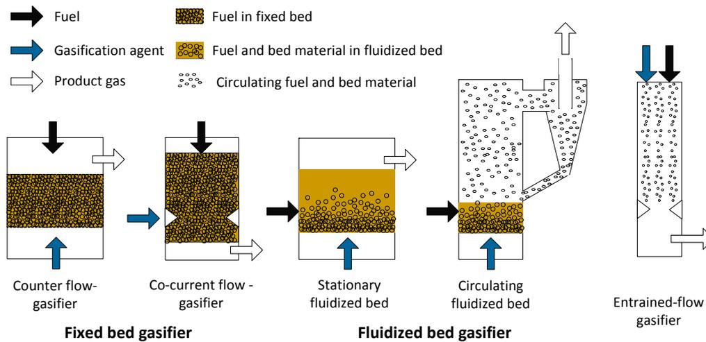
Figure 2: Different types of gasifiers
