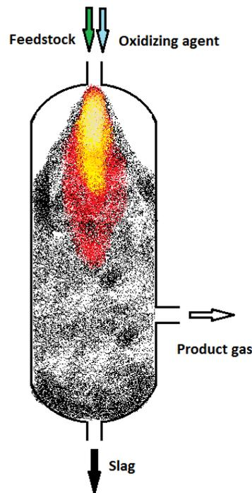
Figure 6: Entrained flow gasifier
