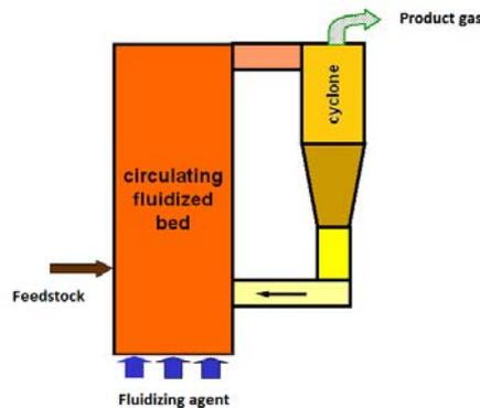
Figure 4: Circulating fluidized bed reactor
