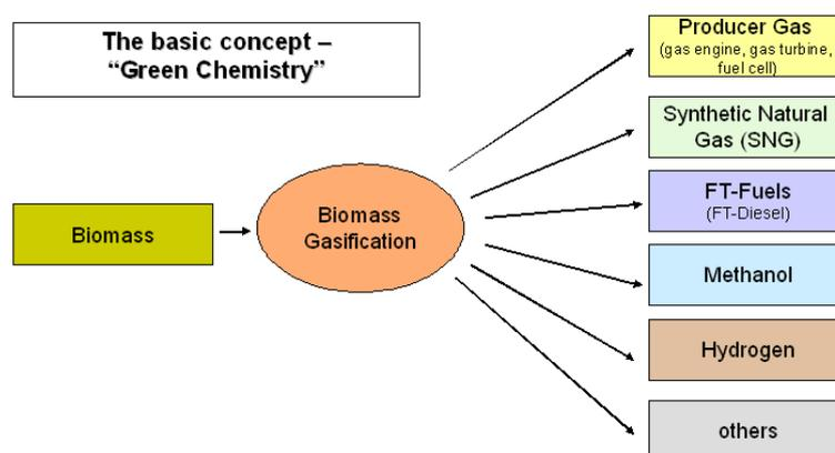
Figure 10: Possibilities of applications of the product gas from FICFB Güssing
