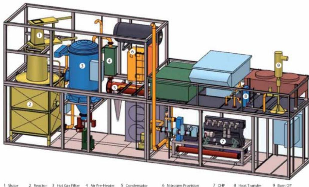
Figure 25: Urbas gasification of biomass – container form
