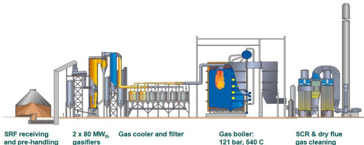
Figure 16: Lahti waste gasification plant
