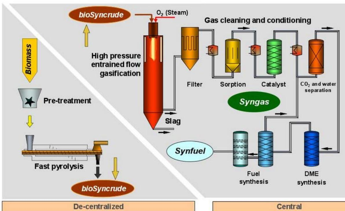
Figure 21: The bioliq process
