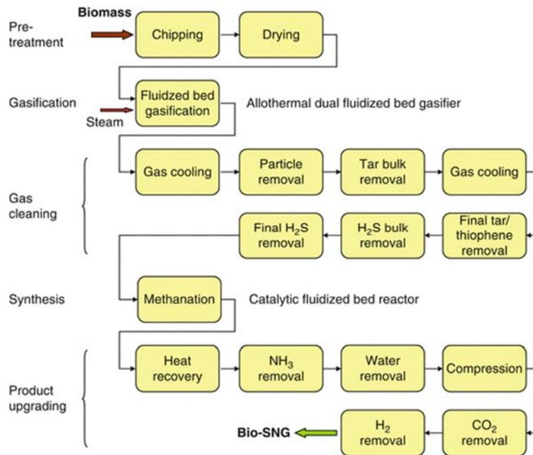
Figure 8: Example of process chain for Bio-SNG production
