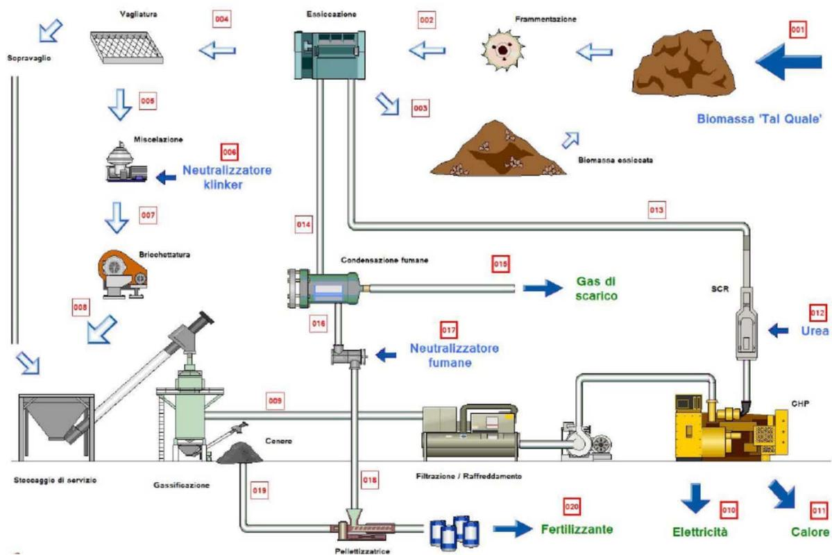
Figure 10: Gasification unit and process diagram
