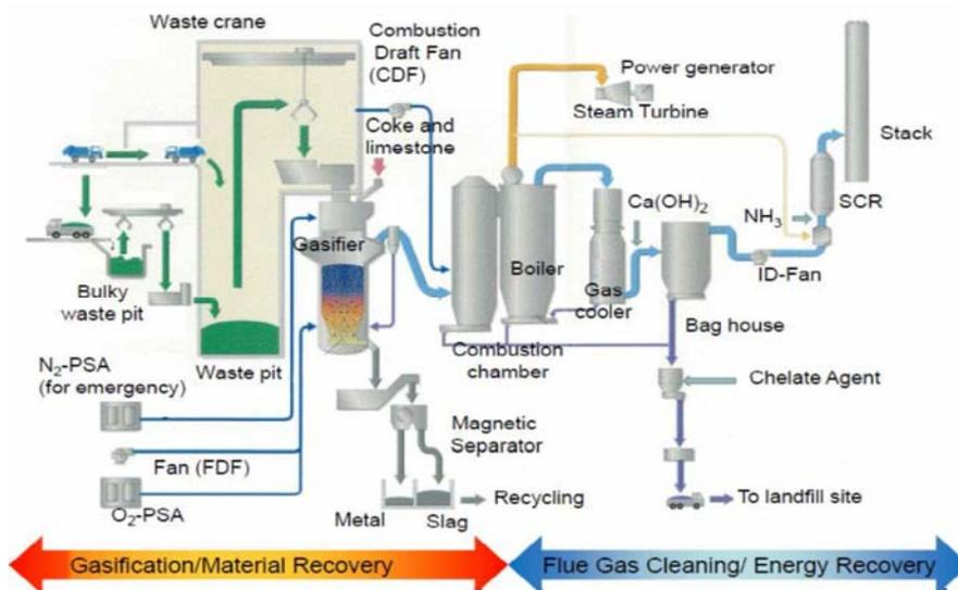
Figure 1: Nippon Steel & Sumikin engineering Co. Ltd. Shaft furnace
