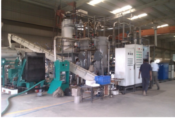
a) 70 KWe downdraft twin-fire gasifier
