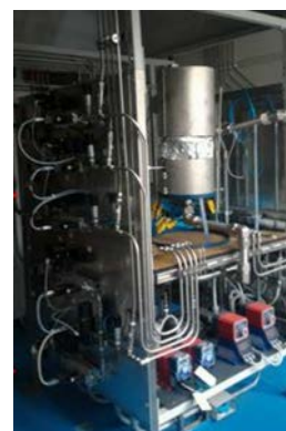
d) Pilot test plant (Inlet syngas flow range: 10–50 Nm 3 /h)
