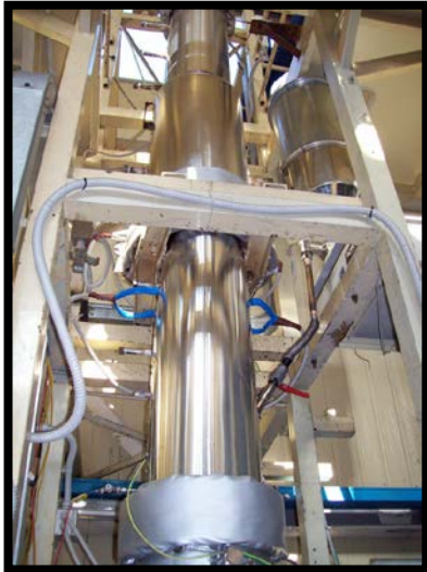
a) 50 kWth Bubbling Fluidized bed gasifier
