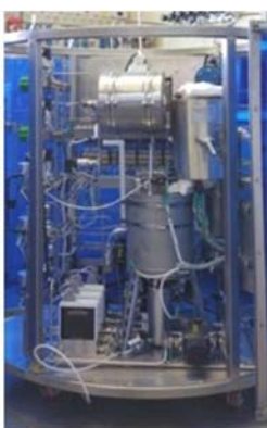
c) Bench scale test plant (left), reformer (right) - Inlet flow range: 1–10 Nm 3 /h.
