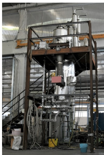
Figure 12. 100 kW th dual bubbling fluidized bed gasifier new version
