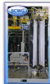
6) Bench scale facilities: 10 kW th gasification plant for tests; Test rig for BioSNG synthesis; Test rig for supercritical water gasification (SCWG);
