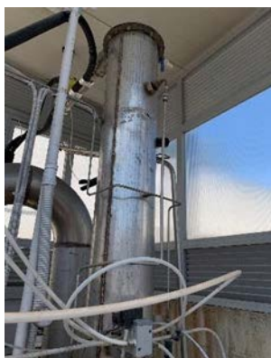
a) Fixed bed Gasifier (updraft) 25 kWt equipped with clean-up gas systems
