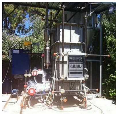
Figure 13. 100 kW th dual bubbling fluidized bed gasifier previous version
