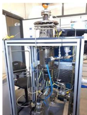
c) Bench scale test plant (left), reformer (right) - Inlet flow range: 1–10 Nm 3 /h.
