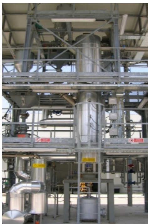
Figure 23. Main design and operating parameters of the pilot scale bubbling fluidized bed gasifier
