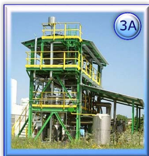
3A) Air/Steam-Blown Updraft Fixed Bed Gasification Plant (150 kW th ) with Wet Gas Cleaning: Bio-Diesel Scrubber coupled with Coalescent Filters. 3B) Scheme of reactor.
