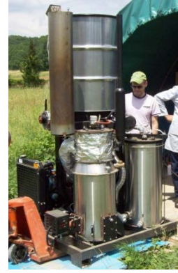
b) 10 kWe downdraft Imbert-type gasifier
