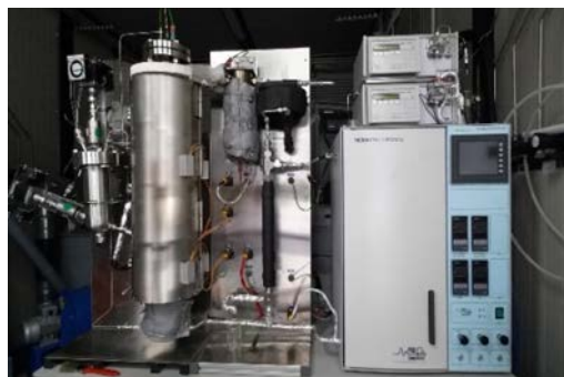
b) Bubbling fluidized bed gasification plant 1,5 kWt
