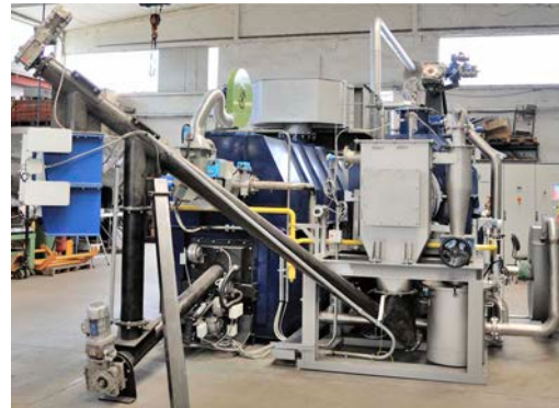
d) 100 kg/h indirectly-fired rotary kiln biomass carbonization unit
