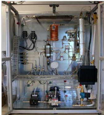
c) Test rig for syngas conversion into bioSNG
