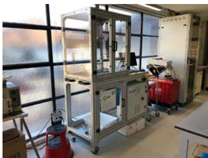
Figure 17. HTC reactor. The reactor allows directly measuring and characterizing in a semi-continuous way the hydrochar and both the liquid and gaseous phases during HTC process. It consists of a 4 liters reactor equipped with an external vessel into which it is possible to extract small amounts of these three phases, without having to wait for the system to be cooled down.
