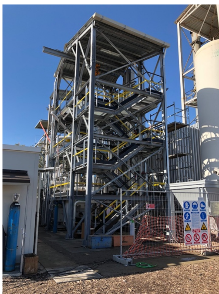
Figure 21. Pilot-scale bubbling fluidized bed unit (500 kW th )
