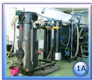
1A) Air-Blown Downdraft Fixed Bed Gasification Plant (120 kW th ), with Conventional Gas Cleaning: Filtration Units and Water Scrubber, combined to Internal Combustion Engines (30-80 kW e ). 1B) Scheme of reactor.
