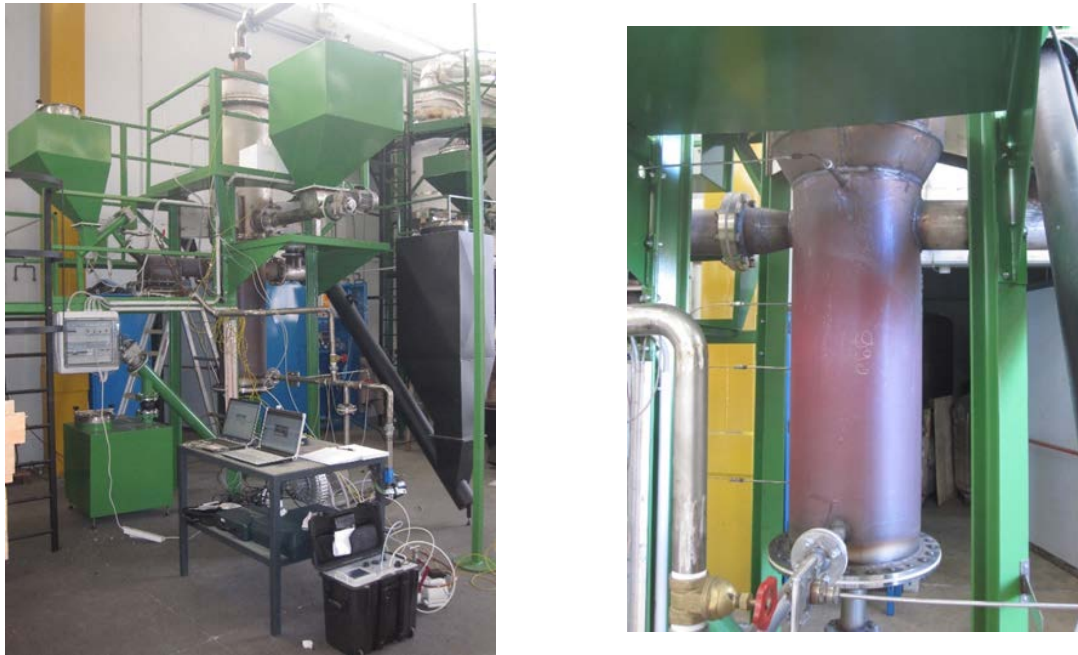
Figure 9. 200 kWth fluidized bed gasifier realized by the spin-off of the University of Teramo
