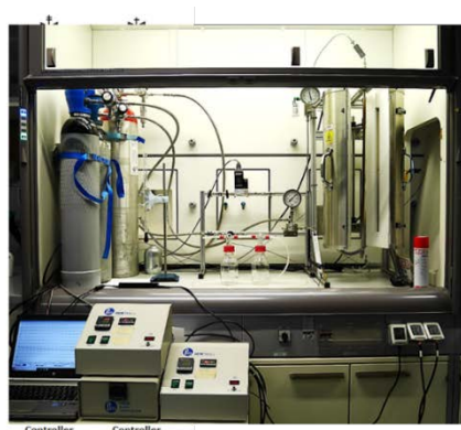
Figure 18. Fischer-Tropsch synthesis & reforming reactor. The catalyst is placed in a fixed bed tubular reactor that is heated with a split-tube furnace controlled with the use of a thermocouple located in the center of the reactor. Gaseous products are analyzed by an on-line gas chromatographer, while products collected in the trap are analyzed off-line by a GC-FID.
