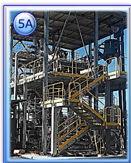
5A) Multi-stage air/steam gasification plant (500 kW th ) with separate plug flow pyrolysis, partial oxidation of tars (vortex combustion), downdraft gasification and syngas filtration on char bed. 5B) Scheme of gasification reactor (3) .
