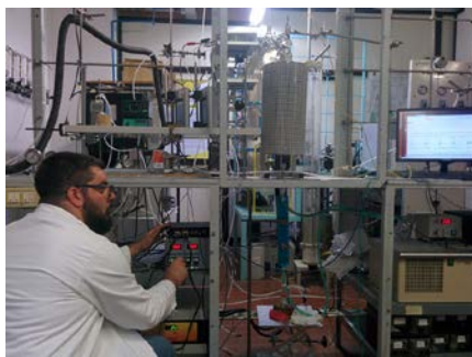
Figure 11. Micro-reactor for experimental test with catalysts and sorbents to be coupled with the gasification process
