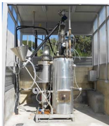
a) Fixed bed Gasifier (updraft) 25 kWt equipped with clean-up gas systems
