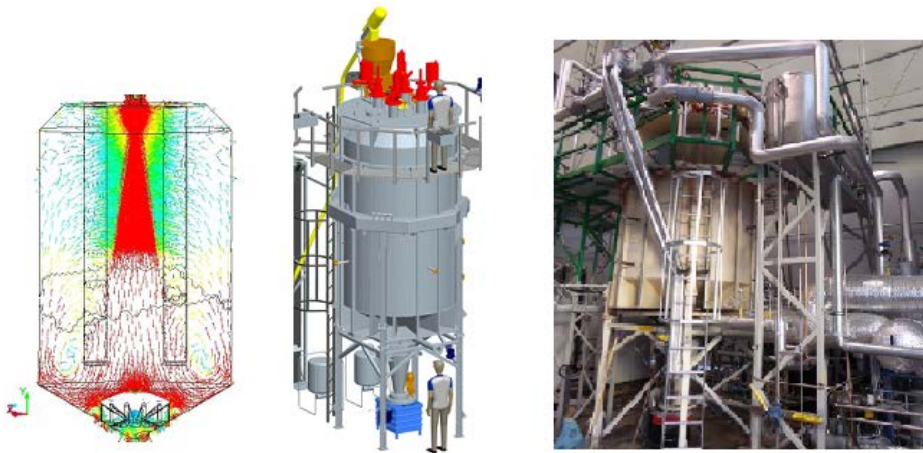
Figure 16. Cortus 500 kW prototype gasifier at Köping; CFD and 3-D models, IRL.
