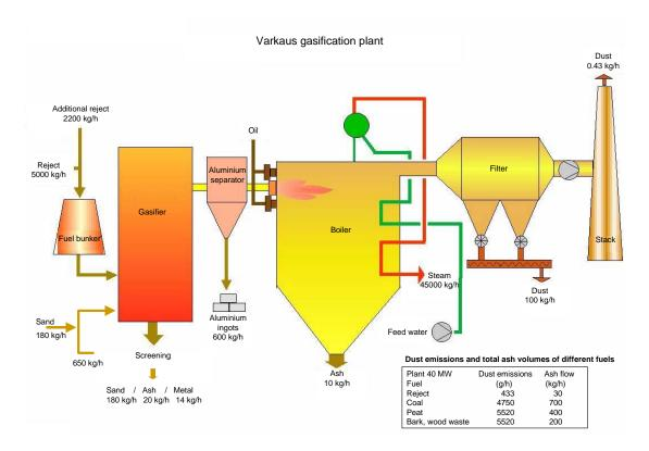
In Corenso's gasification plant, the fibre material in multi-layer packages is recycled in coreboard, the aluminium being recycled as raw material for foil. The remaining plastic is gasified to create energy. The metal and packaging bands in the loads of collected raw material are sent to the metal industry for recycling. Thus, everything is recovered.
