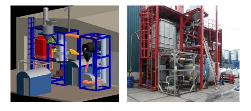
Figure 8: The Synvalor pilot gasifier
