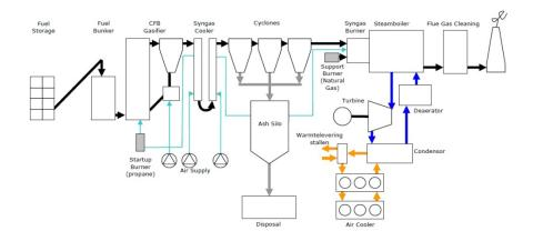
Figure 13: HoSt gasification system for difficult fuels with CFB gasifier and syngas boiler
