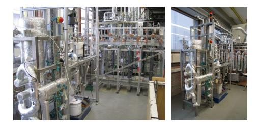
Figure 16: Lab-scale bioSNG test facility coupled to lab-scale MILENA gasifier and OLGA tar removal
