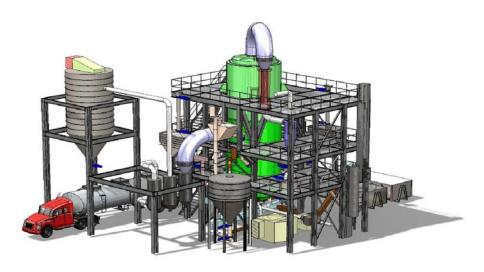
**Figure 12**: The 11.6 MW waste wood demonstration plant in Alkmaar with bioSNG slip-stream, expected to be started late-2014
