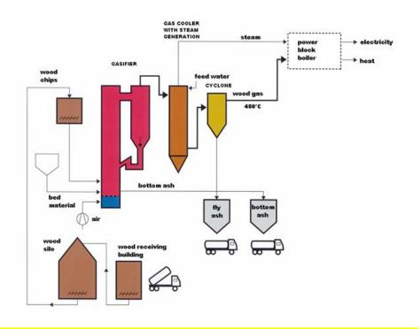
Figure 3: The system of the Essent 85 MW waste wood gasifier for indirect co-firing
