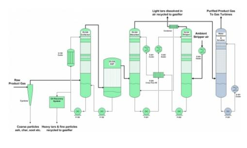
Figure 6: Schematic OLGA process for tar and particles removal
