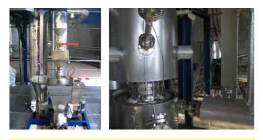
Figure 18: The 100  $kW_{th}$  biomass gasification test facility of Delft University (left) and high-temperature filter (right)
