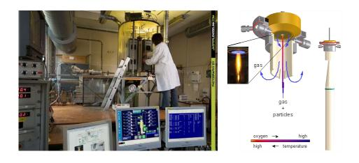
Figure 17: The LCS test facility to simulate Entrained Flow gasification
