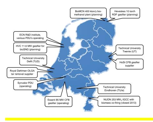
Figure 1: Biomass gasification in the Netherlands
