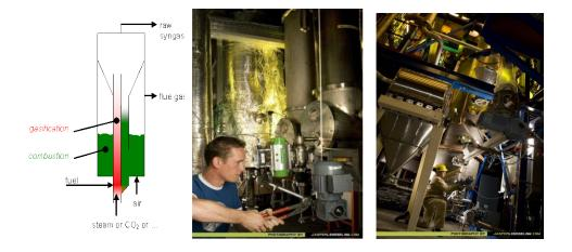
**Figure 15**: MILENA gasification technology at ECN: the technology scheme (left), 25 kW test facility (centre), 0.8 MW test facility (right)
