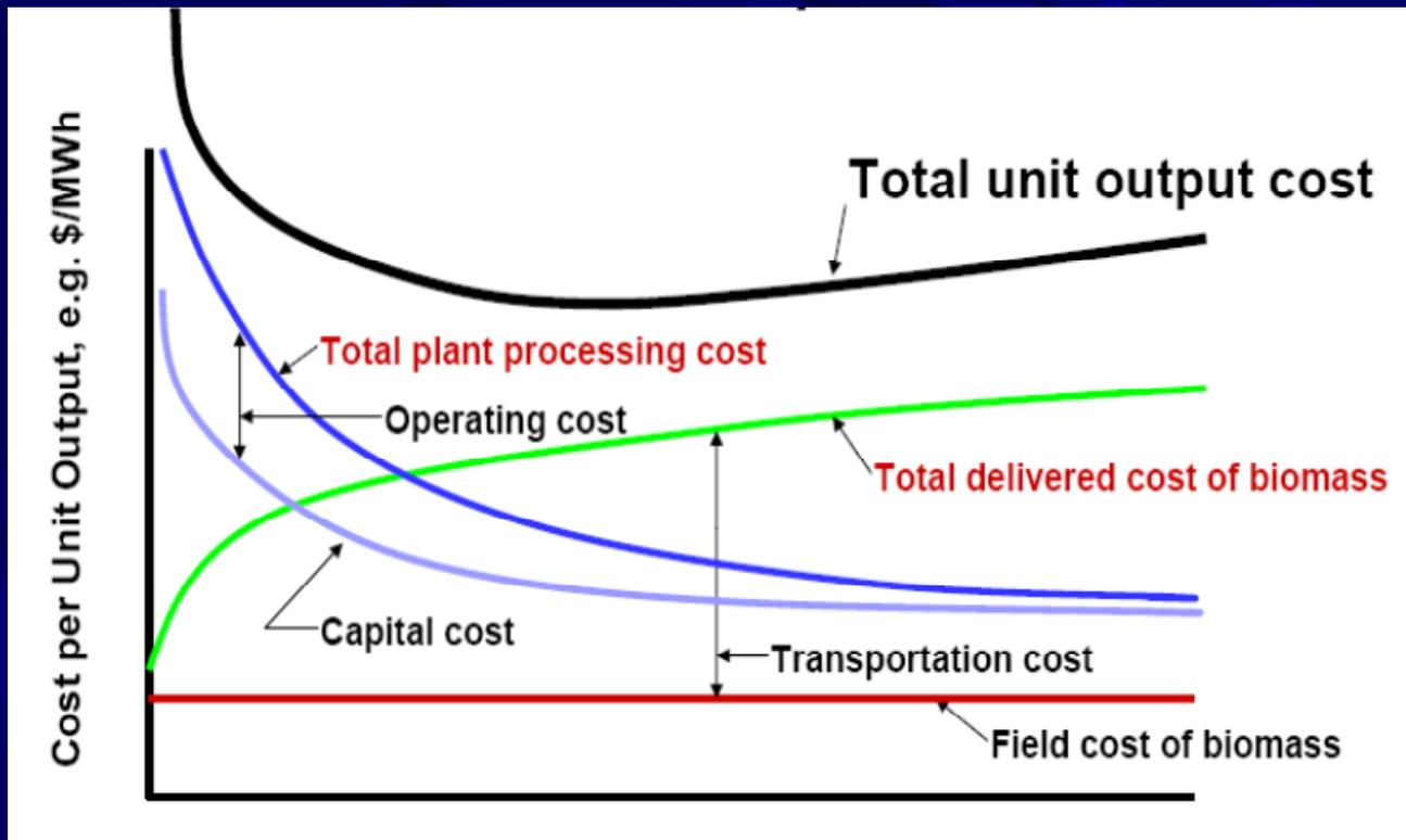
▲ Capital cost and operation cost for unit energy output are reduced with the plant scale. However, cost of biomass delivered to the plant increases with the plant scale.
