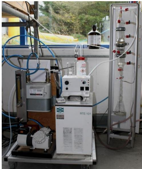
Figure 51. Petersen column applied during measurement campaign at the 100kW<sub>th</sub> LT-CFB gasifier. Picture courtesy of DTU.
