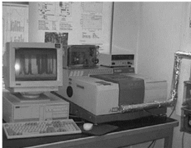
Figure 13. FTIR equipment applied by Technical University Delft [22].
