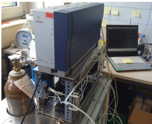
Figure 17. Micro-GC unit (GC-TCD) used for online analysis of H<sub>2</sub>S and COS trace concentrations as well as bulk gases. Picture courtesy of PSI.
