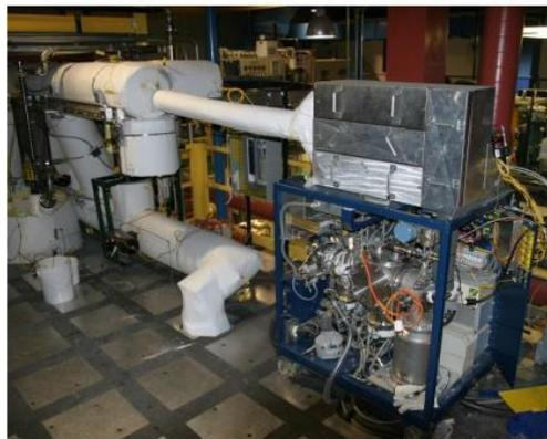
Figure 41. Molecular Beam Mass Spectrometer developed by NREL: formation of molecular beam (left), transportable MBMS apparatus (right) [89].
