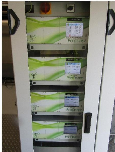
Figure 46. Set of 4 laser spectroscopy OF-CEAS in the shelter of the GAYA Platform. Picture courtesy of ENGIE Lab CRIGEN.
