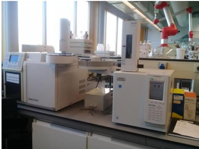
Figure 20. GC-FID unit used for tar analysis. Picture courtesy of ECN part of TNO.
