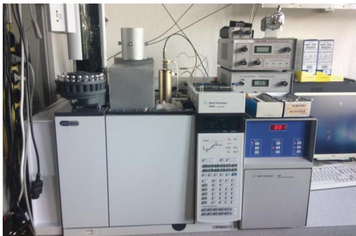
Figure 23. Stand-alone SCD (with no preceding chromatography column) used at PSI for total sulphur measurements. Images courtesy of PSI [10].
