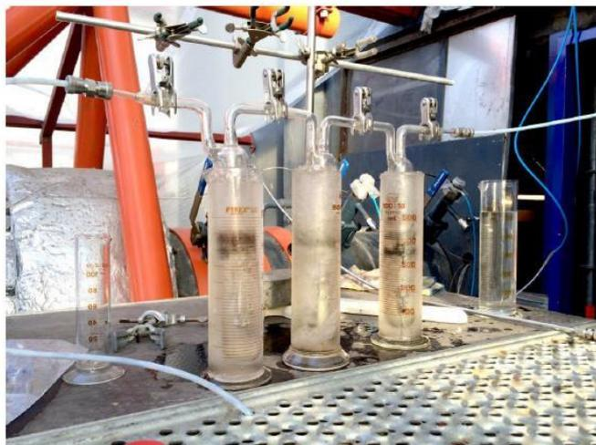
Figure 77. Impinger train used by DTU for determination of total nitrogen content in the gas [135].
