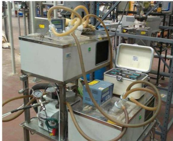
Figure 64. Tar sampling system used at CIEMAT [130].
