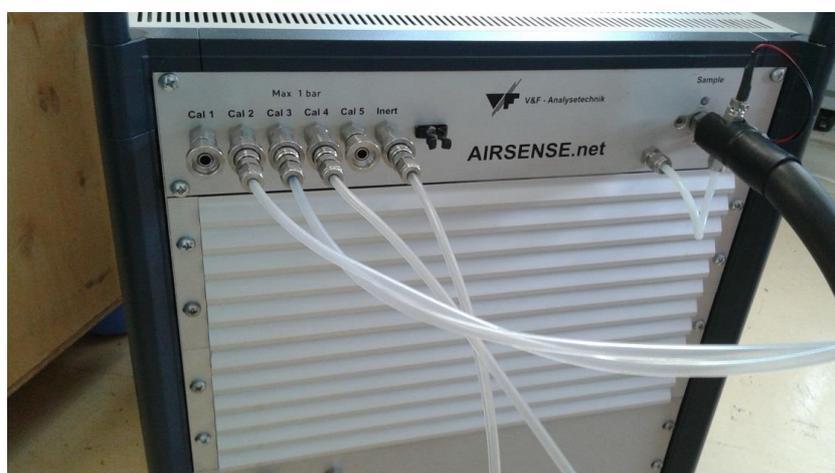
Figure 24. IMR-MS (Ion Molecule Reaction Mass Spectrometry). Picture courtesy of CEA.
