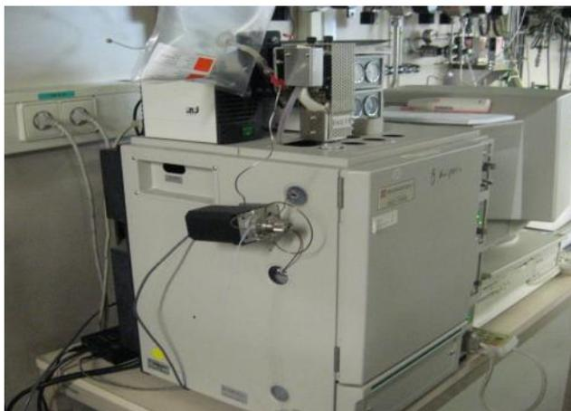
Figure 21. GC-FPD unit at ECN part of TNO for analysis of S-compounds.
