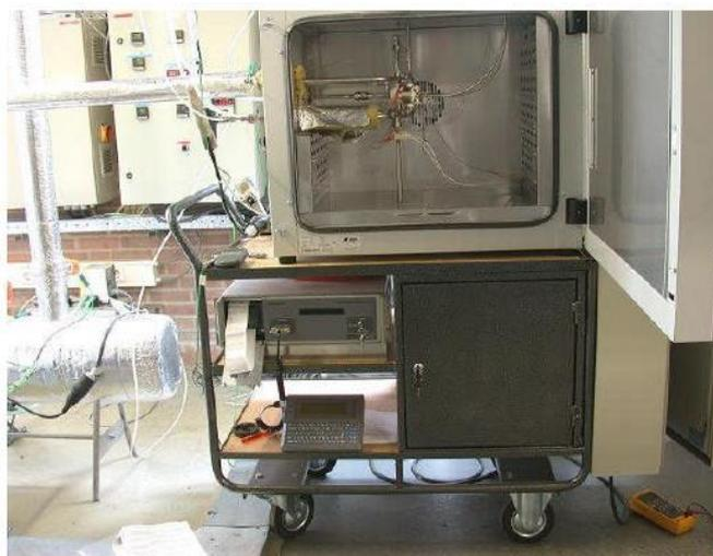
Figure 70. The tar dew point sensor located in the oven for testing [141] .
