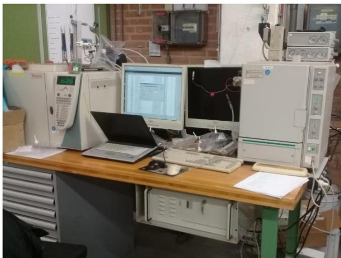
Figure 22. GC-FPD (right) and GC-FID equipment for measurement of sulphur compounds and C<sub>1</sub>-C<sub>6</sub> hydrocarbons, respectively. Courtesy of ECN part of TNO.
