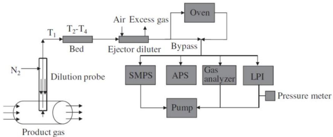
Figure 49. Schematic implementation of particle measurement system in CFB and indirect BFB by Linnaeus University [143].
