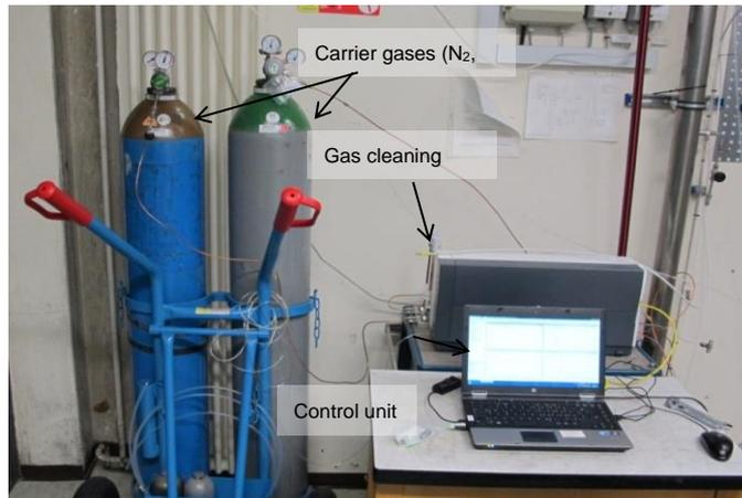
Figure 81. Micro-GC analyser at REGA setup [159].
