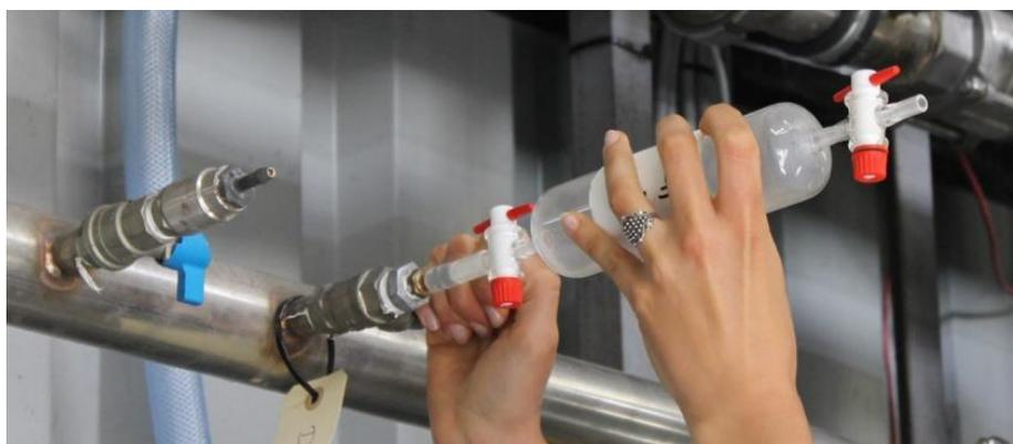
Figure 5. Gas sampling with gas pipettes for permanent gases + GC-TCD (offline) analysis at DTU [11].
