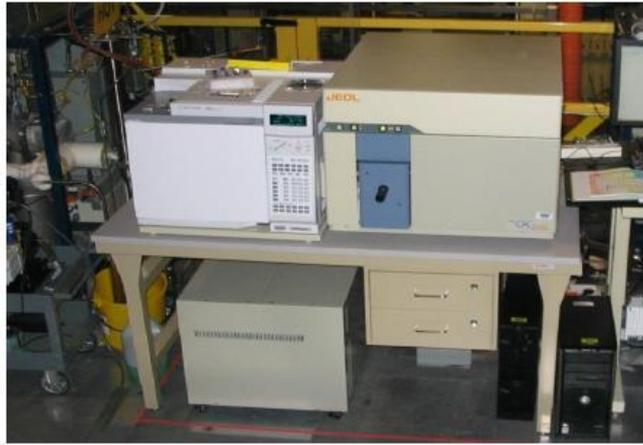
Figure 113. High-resolution mass spectrometer installed at NREL laboratories [61].
