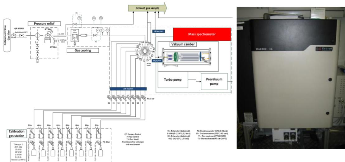
Figure 64. Mass spectrometer used at the Bioliq plant by KIT: schematic setup and picture [159].
