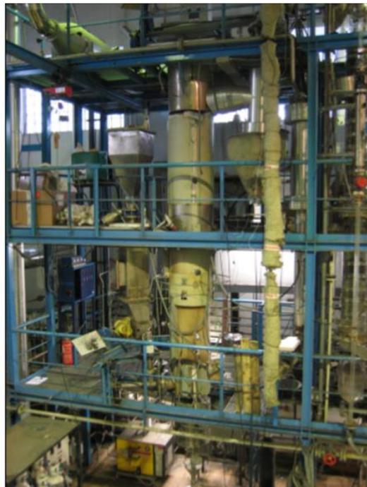
Figure 88. View of the 100 kW<sub>th</sub> BFB pilot plant located at University of Seville [85].
