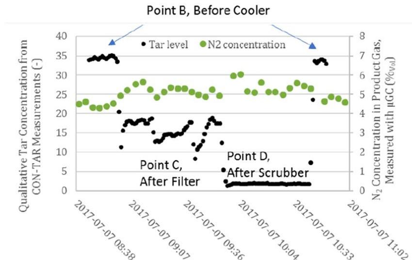
Figure 105. Results of testing of CON-TAR prototype at GoBiGas plant for qualitative online measurement of total tar content [60].
