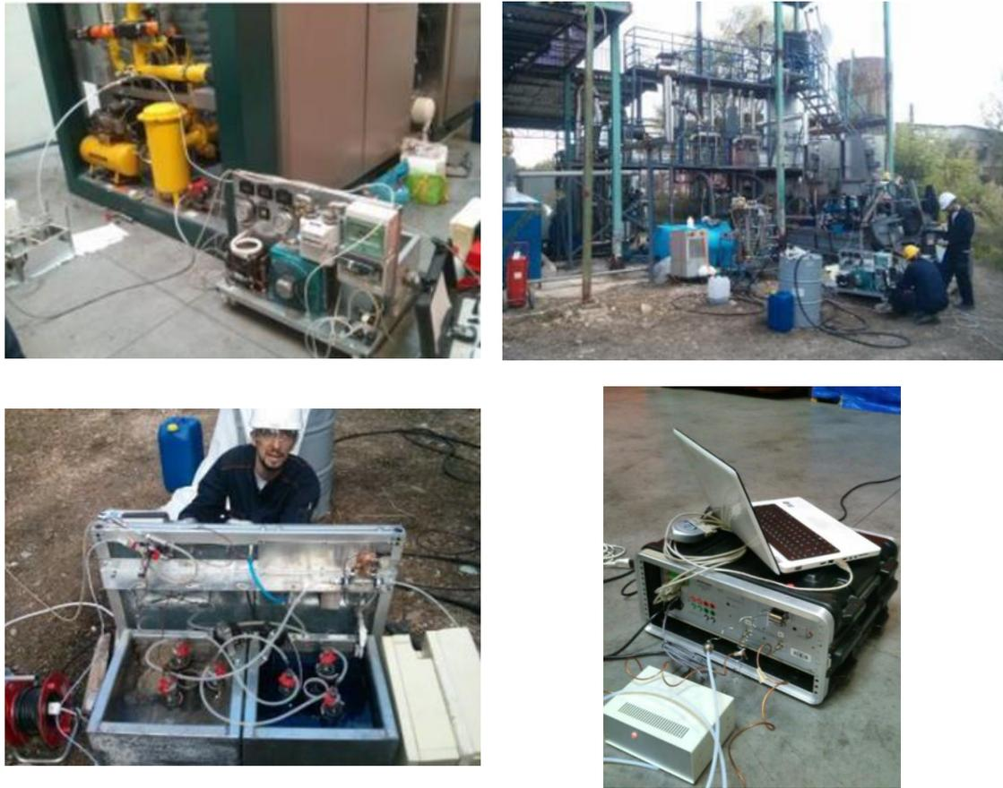
Figure 85. Gas analysis at measurement campaign by RE-CORD and UNIBZ in small-scale gasification plants [175][176].
