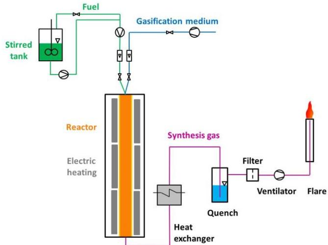
Figure 79. Picture and process flow scheme of the REGA bench-scale gasifier [159].
