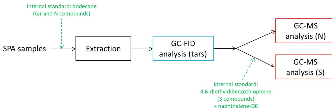
Figure 29. Procedure developed by ECN part of TNO for the extraction and analysis of SPA samples for determination of tars, and S- and N- organic compounds.
