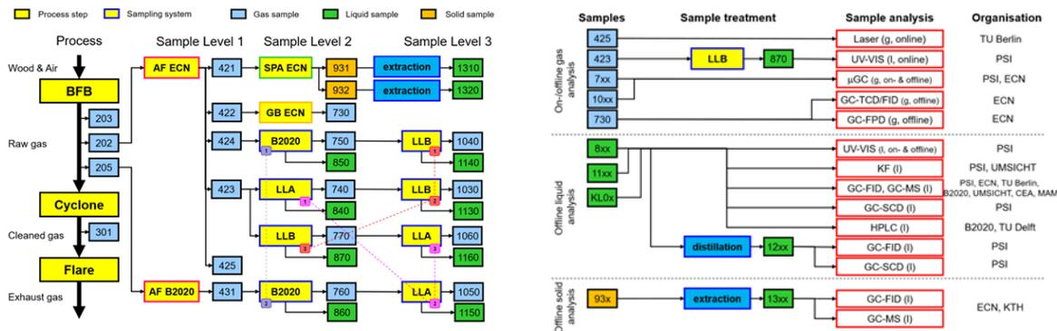
Figure 115. Configuration (left) and sample treatment (right) during gas analysis round robin campaign at PSI, November 2013 [225].
