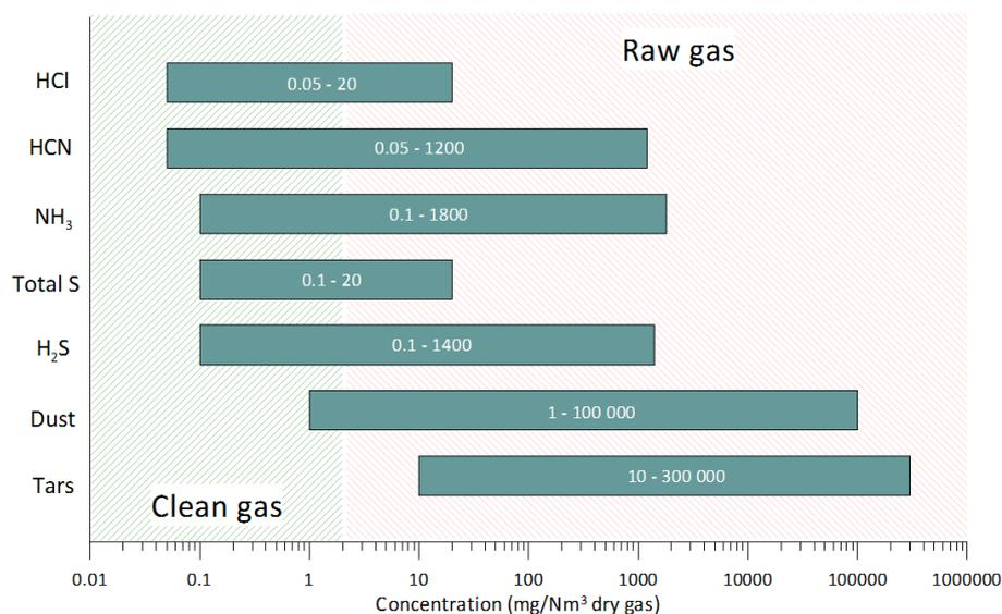
Figure 1. Typical concentrations of contaminants in product gas (adapted from [4]).
