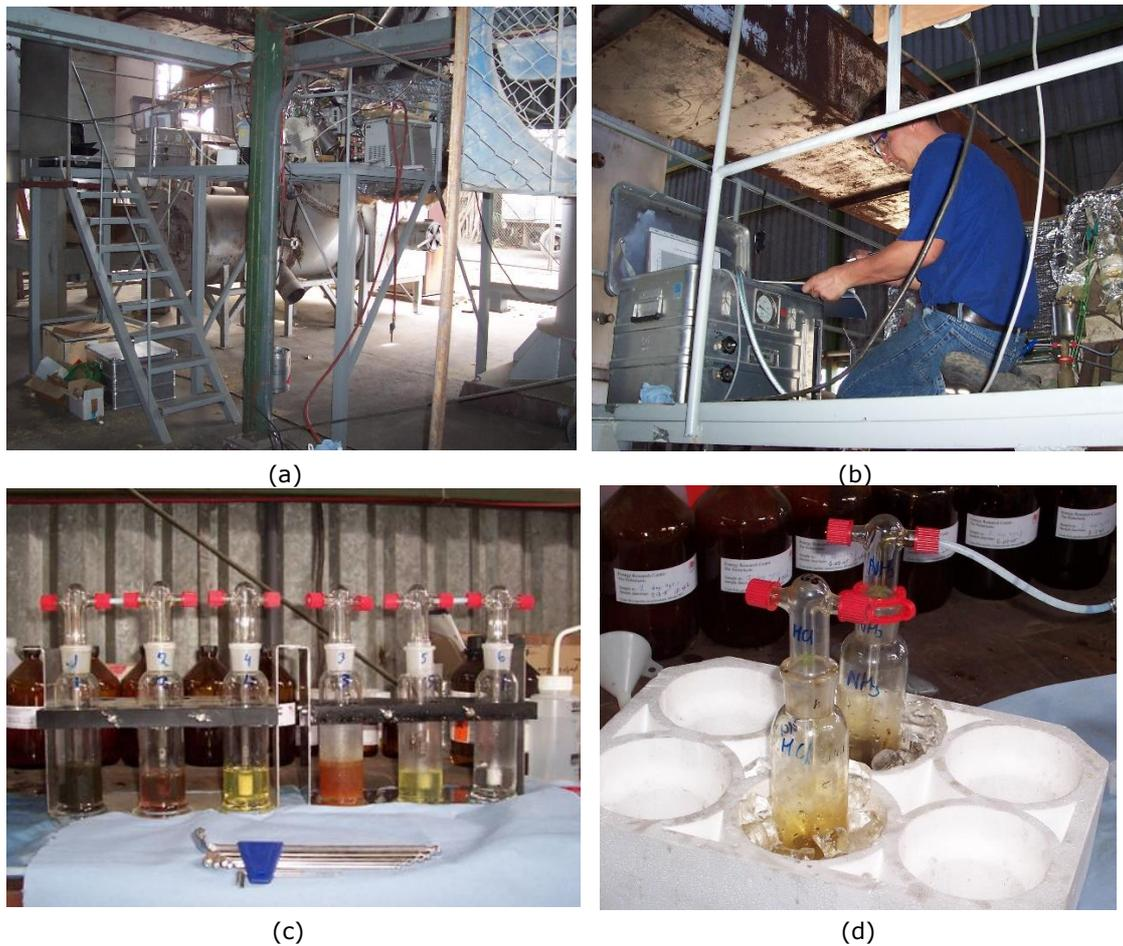
Figure 73. Measurement campaign at Costa Rica gasification plant: gasification plant (a); operating the gas analysis train (b); impinger train after gas sampling for tar measurement (c); impingers for wet chemical analysis after gas sampling (d). Pictures courtesy of ECN part of TNO.
