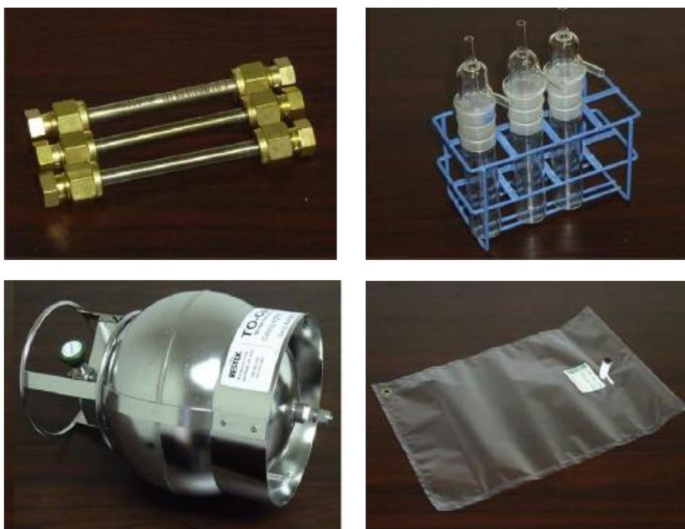
Figure 38. Available methods for sampling of siloxanes from biogas [138].
