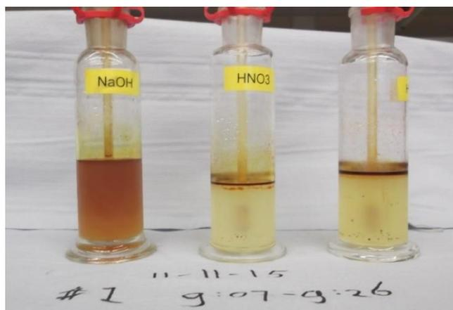
Figure 26. Solutions contained in impingers after gas sampling for offline measurement of  $\text{NH}_3$  and  $\text{HCN}$ . Picture courtesy of ECN part of TNO.
