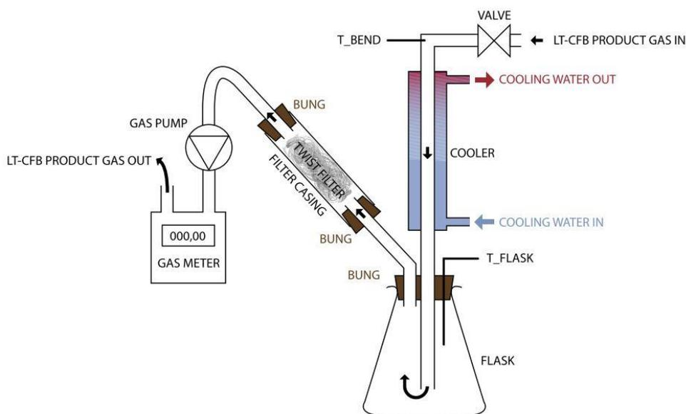
Figure 12. Tar and water condensation setup applied by DTU [24].
