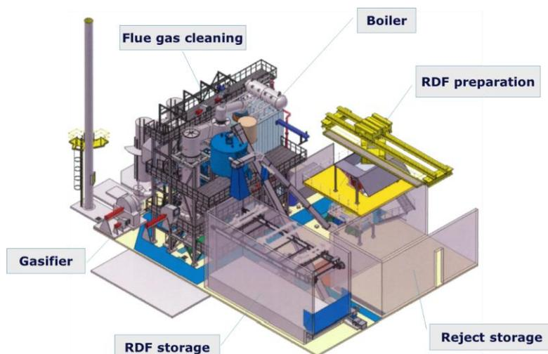
Figure 74. Schematics of the ESKA paper rejects gasification plant [169].
