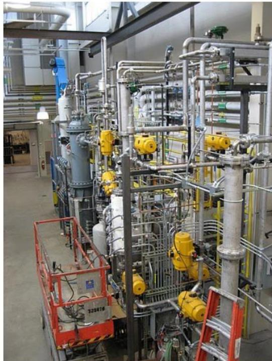
Figure 83. The complete Iowa State University 25 kg/h gasifier and cleaning system [172].
