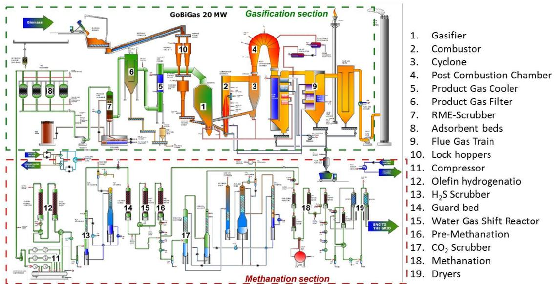
Figure 53. Schematic of GoBiGas plant [60].
