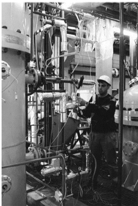
Figure 78. Pressurized fluidized bed setup at Technical University Delft [79].
