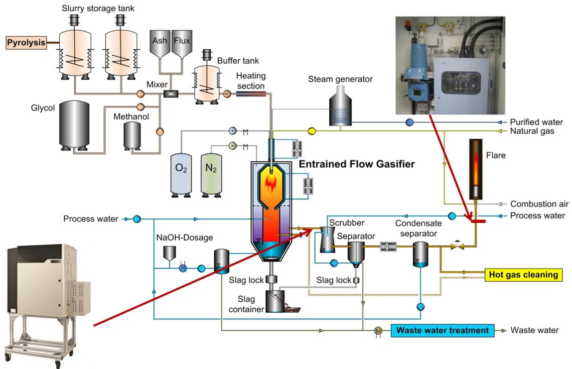
Figure 62. Flowsheet of Bioliq entrained flow gasifier pilot plant with sampling points for gas analysis [159].
