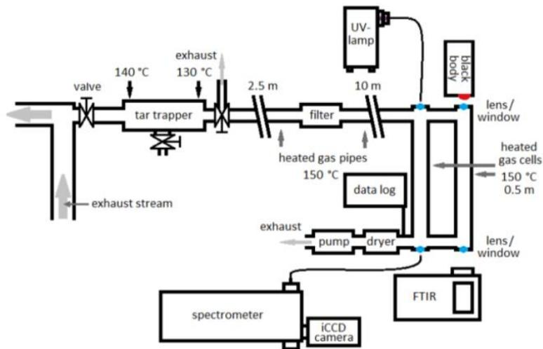
Figure 109. Gas sampling system used by DTU for online UV/IR measurement of tars and other gas compounds [11][65][219].
