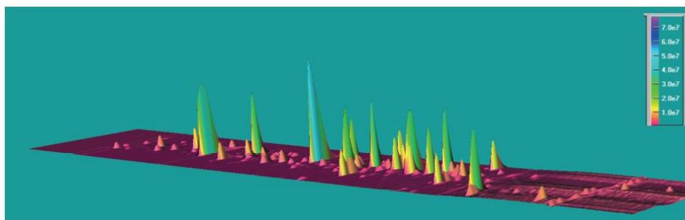
Figure 60. 3D-chromatogram obtained by ENGIE Lab CRIGEN and ESPCI Paris Tech from product gas from an agricultural biomass [81].
