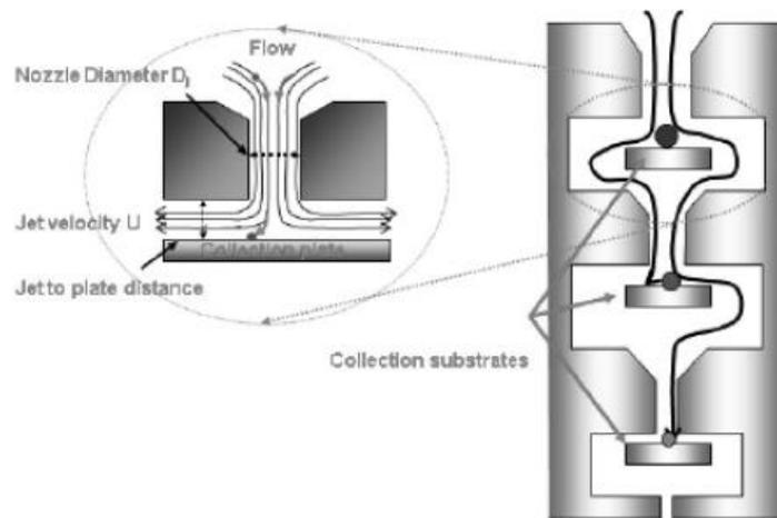
Figure 44. Schematic of gas and particles flow along the stages of the cascade impactor [141].
