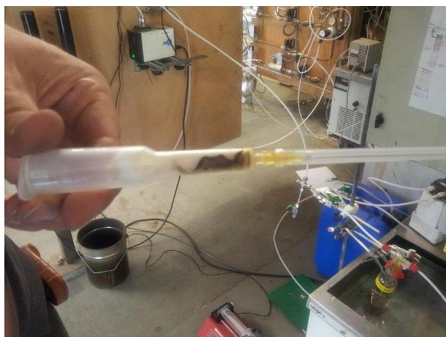
Figure 13. Measurement of water using  $P_2O_5$  – effect of sampling tar-containing gas. Picture courtesy of ECN part of TNO.
