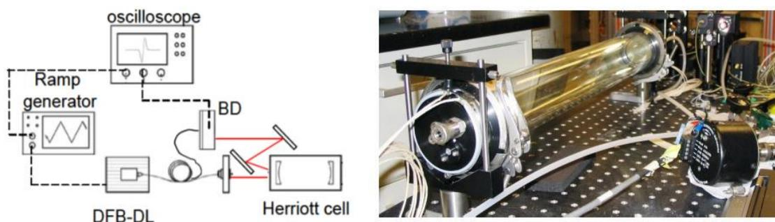
Figure 111. Diode laser spectroscopy developed by NREL: BD – balanced detector, DFB-DL – distributed feedback/ diode laser [61].
