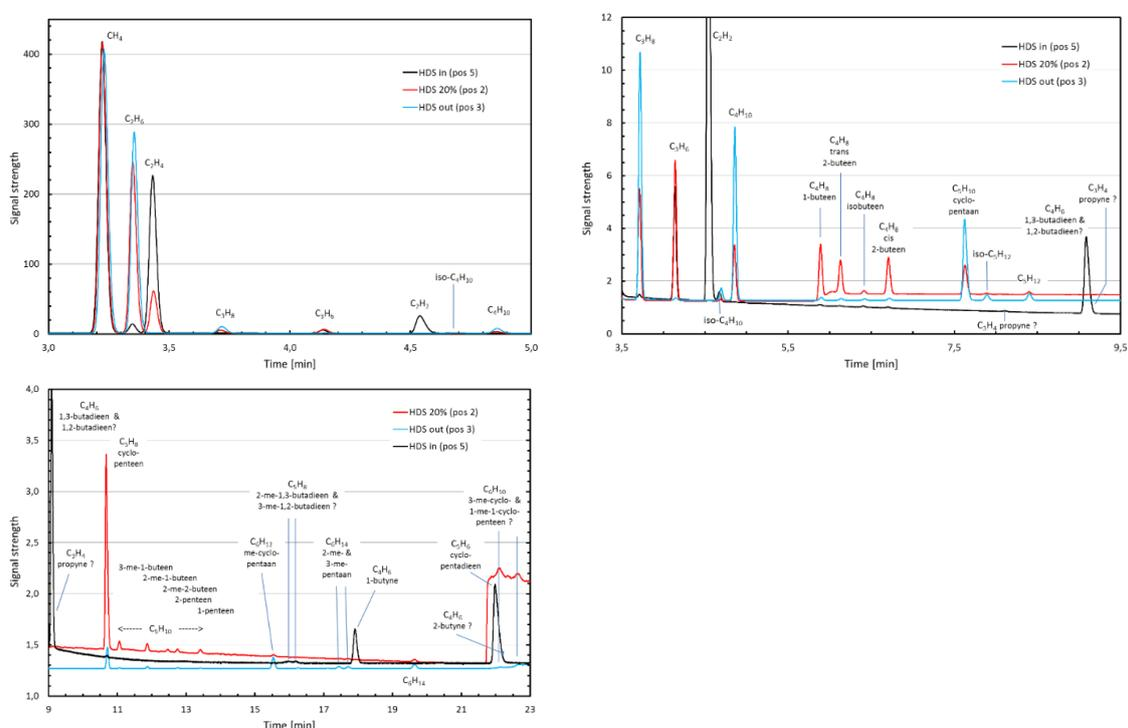
Figure 6. Fate of C<sub>1</sub>-C<sub>5</sub> hydrocarbons in HDS reactor using GC-FID analysis. Gas analysis positions: inlet HDS reactor (black line); 20% within the HDS catalyst (red line); outlet of HDS reactor (blue line). Figures courtesy of ECN part of TNO.
