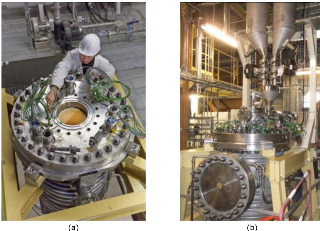
Figure 96. Entrained-flow reactor (GIROFLE) at CEA Research Centre: (a) top of the reactor; (b) fuel powder injection. Pictures courtesy of CEA.
