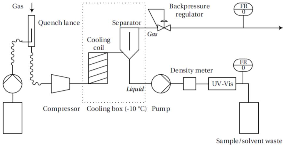
Figure 18. Schematic layout of the quench sampling system (coupled to online UV-Vis spectroscopy analysis) developed by PSI for online tar analysis [63].
