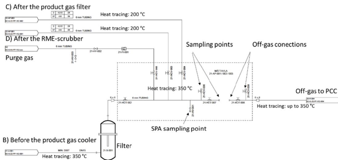
Figure 54. Schematic layout of new gas sampling system implemented at the GoBiGas plant [60].
