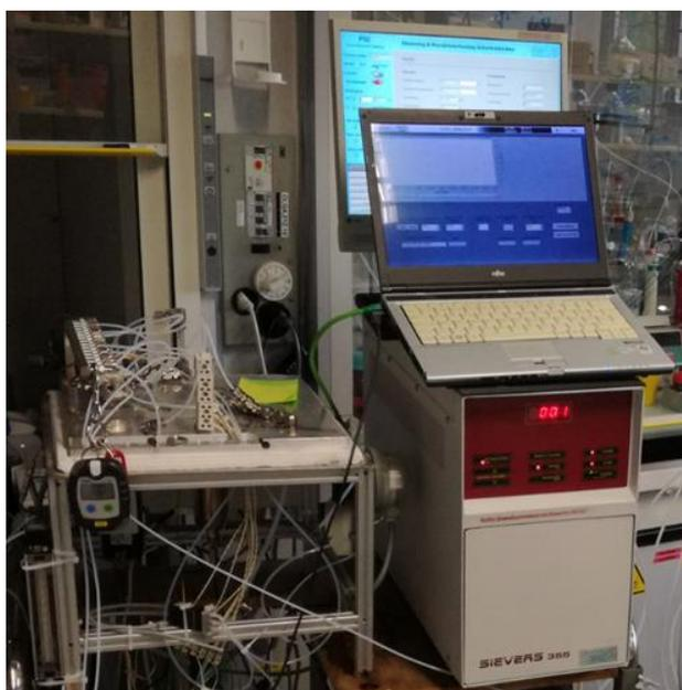
Figure 24. Stand-alone SCD (with no preceding chromatography column) used at PSI for total sulphur measurements. Picture courtesy of PSI.
