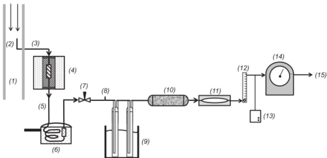
Figure 11. Gas conditioning and gas sampling system used at Iowa State University [22].
