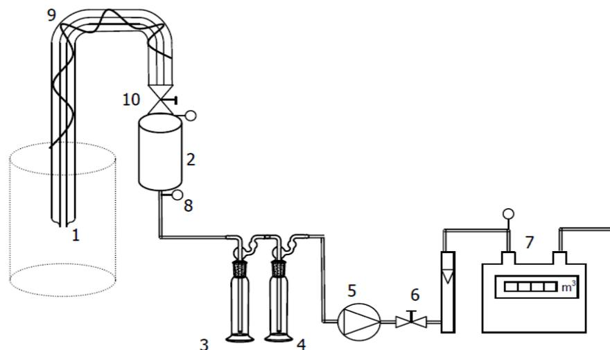
Figure 46. Implementation of measurement of particulate matter in gasifier setup using a cascade impactor by TU Delft [69]: 1. Sampling probe; 2. Cascade impactor; 3. and 4. Condenser and silica flask for trapping of water and tars; 5. Gas pump; 6. Rotameter for flow regulation; 7. Gas meter; 9. Electrical heating; 10. High-temperature valve.
