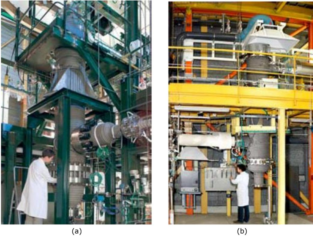
Figure 94. Gasification pilot plants at CEA: (a) High-temperature fluidized-bed (LFHT); (b) High-temperature tar cracker (PEGASE). Pictures courtesy of CEA.
