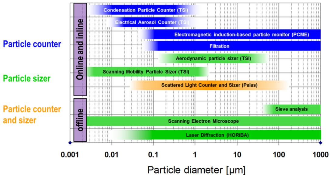
Figure 40. Overview of available methods for measurement and analysis of particulate matter [140].
