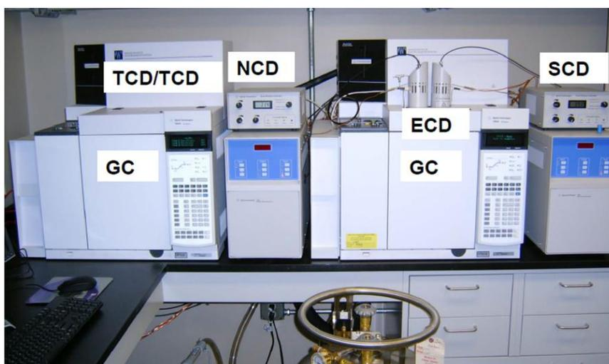
Figure 21. GC equipment applied at Iowa State University for online determination of S- and N compounds (including SCD detector for sulphur compounds, NCD detector for nitrogen compounds, and ECD for nitrous oxide) [76].
