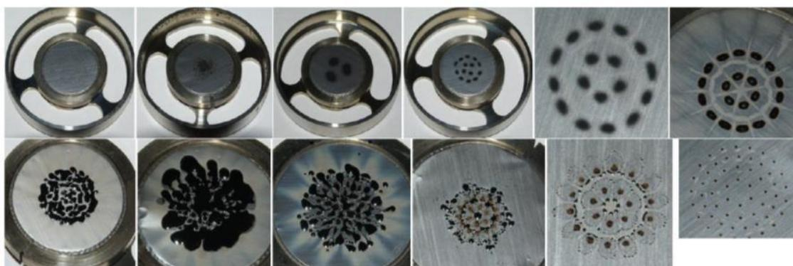
Figure 48. Stage plates of low-pressure impactor after sampling of particles from product gas at 160°C (Abo Akademi University, [69]).
