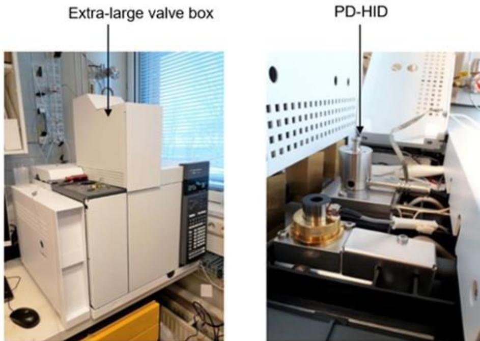
Figure 4. GC-TCD/FID/PDHID unit used at VTT for offline gas analysis [12].
