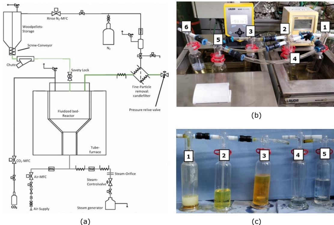
Figure 93. (a) Schematic view of the TU Graz gasifier; (b) Tar sampling; (c) Impingers after tar sampling. Pictures courtesy of TU Graz.
