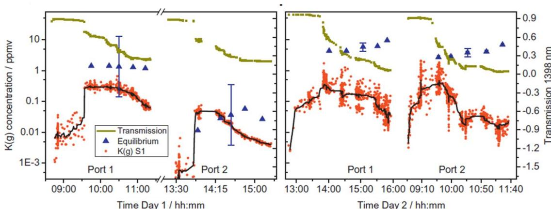
Figure 36. Results of online K measurement using TDLAS: peat (left) and wood (right) as gasification feedstock. Comparison with equilibrium calculations is displayed [15].
