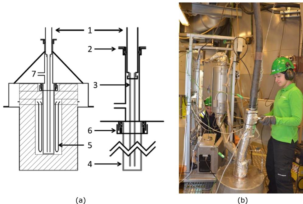
Figure 106. Schematic of the HTR (High-Temperature Reactor) developed by Chalmers for the online determination of C, H, O and N in the product gas [216].
