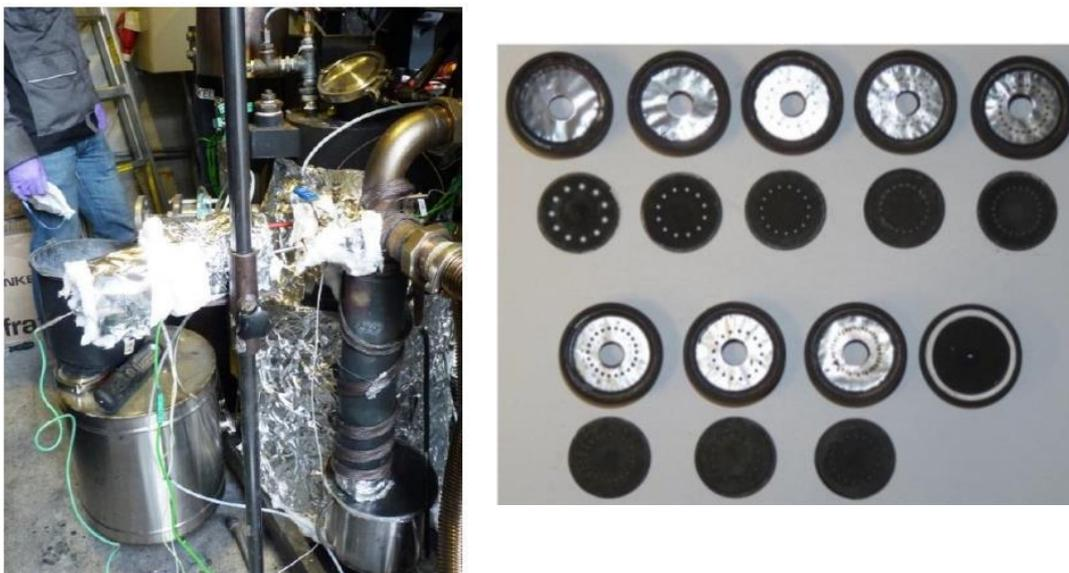
Figure 47. Implementation of high-temperature impactor in product gas line at TU Graz (left); loaded collection plates of high-temperature impactor after measurement (right) [69].
