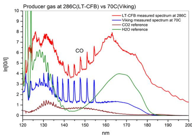
Figure 67. Comparison of optical (UV absorption) in-situ measurement of product gas from Viking (70°C) and LT-CFB gasifiers [122].
