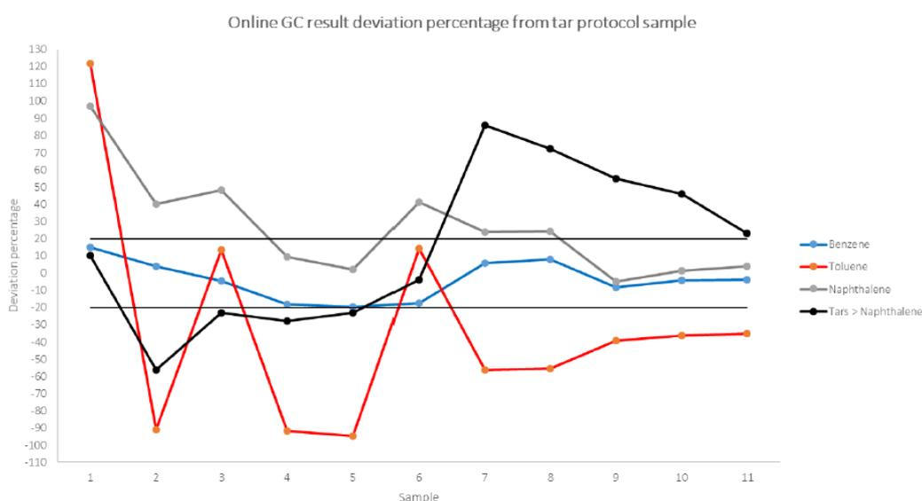
Figure 14. Comparison of results of the online measurement of tar developed by VTT with the tar guideline method [19].
