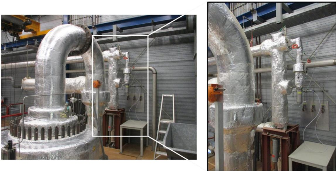
Figure 100. Gas analysis sampling point at outlet of pilot-scale MILENA gasifier. Picture courtesy of ECN part of TNO.
