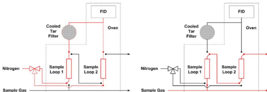
Figure 101. Basic principle of the FID online tar analysis method developed by University of Stuttgart. Left: sampling phase; right: analysis phase [2][19].
