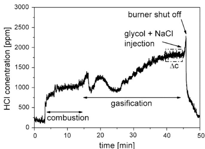
Figure 31. Online measurement of HCl using TDLAS during combustion and gasification [16].
