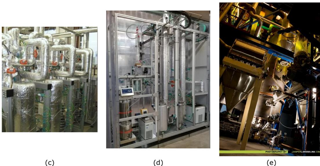
Figure 99. Gasification-related research facilities at ECN part of TNO: (a) WOB BFB gasifier, 5 kW<sub>th</sub> input; (b) MILENA lab-scale indirect gasifier, 25 kW<sub>th</sub> input; (c) OLGA tar removal unit; (d) ESME methanation lab-test rig; (e) BTX scrubbing unit; (f) MILENA pilot gasifier, 800 kW<sub>th</sub> input.
