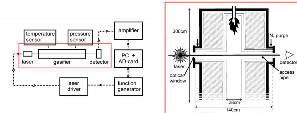
Figure 30. Schematic implementation of TDLAS setup for online measurement of HCl at an entrained-flow gasifier [16].
