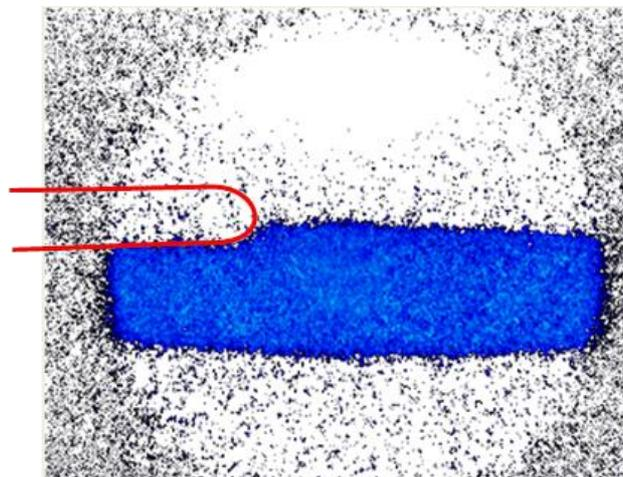
Figure 50. Time-averaged visualization of particle distribution inside the Research Gasifier REGA at KIT using laser-induced fluorescence (LII) [144].
