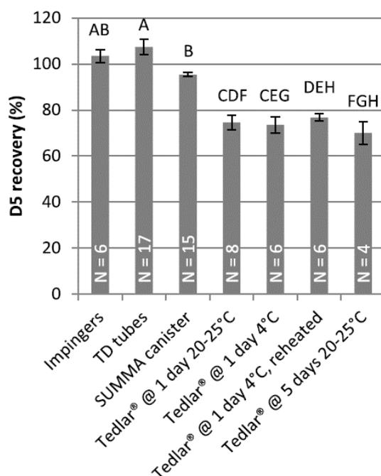
Figure 39. Efficiency of siloxane (D5) recovery using different sampling techniques [138].
