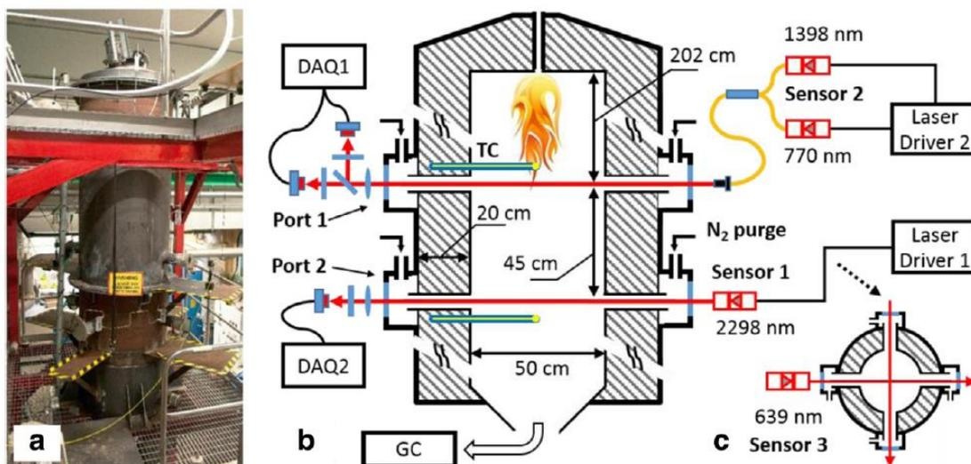
Figure 35. Implementation of TDLAS by Umeå University for online measurement of K, CO, and H<sub>2</sub>O in syngas: (a) 100 kW<sub>th</sub> entrained-flow gasifier at Piteå, Sweden; (b) schematic layout of the implementation of the sensors in the gasifier [15].
