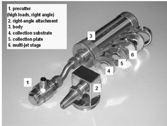
Figure 43. PILAT MARK V cascade impactor used by ECN part of TNO [142].
