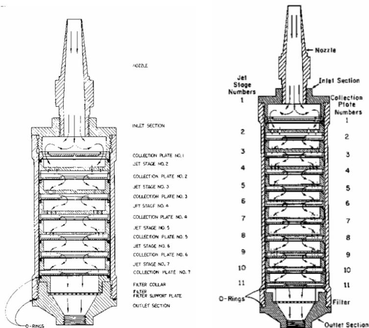
Figure 45. Cross-section of the MARK III (left) and MARK V (right) PILAT impactor [142].
