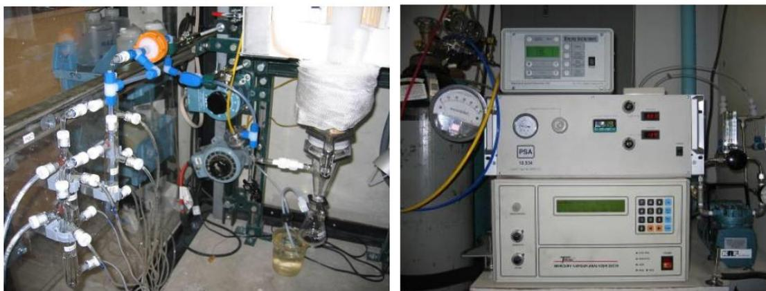
Figure 37. Online measurement of mercury in gas phase by Wendt et al.: schematic layout of sampling and analysis train (top); sampling system (bottom left); cold vapour atomic fluorescence (CVAF) mercury analyser and Hg source calibration system (bottom right) [131].
