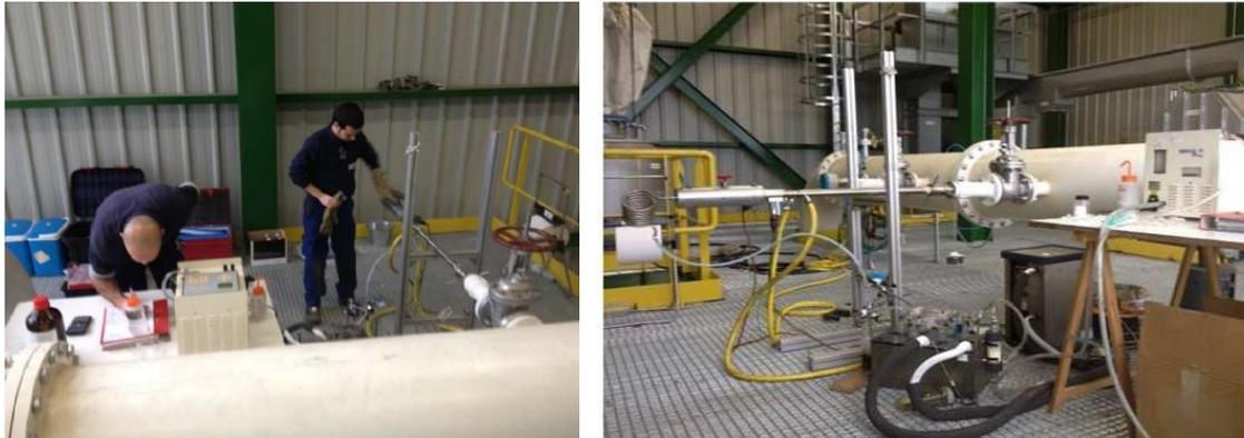
Figure 87. Gas sampling during measurement campaign at CENER (left) and implementation of tar guideline sampling [177].
