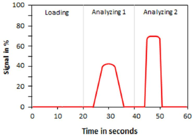
Figure 102. Characteristic peaks derived from FID analysis from the online tar analyser developed by University of Stuttgart. The difference between peak areas corresponds to tar content [2][19].
