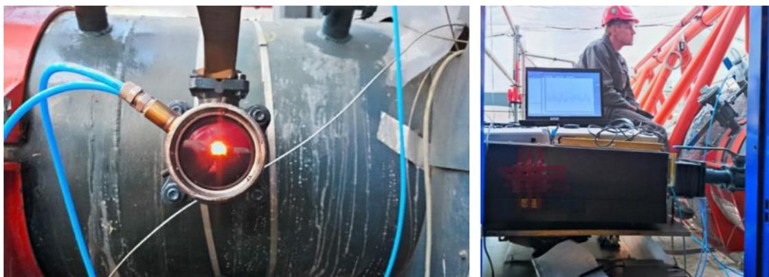
Figure 65. FTIR absorption measurements by DTU at the LT-CFB Pyroneer gasifier [11].
