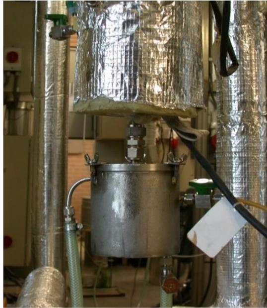
Figure 7. Condensation pot of gas pre-sampling system used at ECN part of TNO [9].
