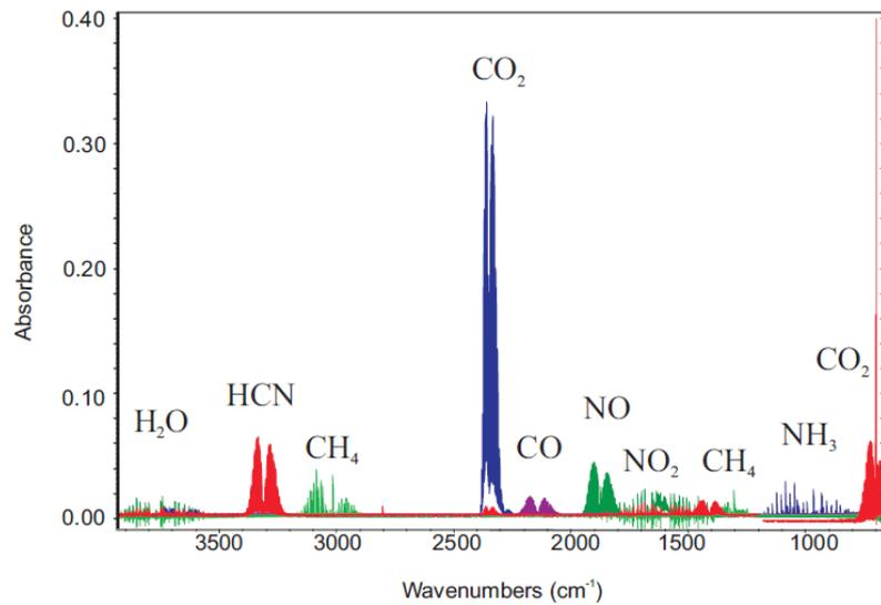
Figure 27. Spectral regions of gases typically present in pyrolysis, gasification and combustion processes [111].
