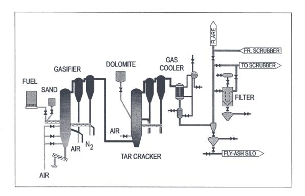
Figure 1. Termiska Processer (TPS) CFB Gasification Pilot Plant
