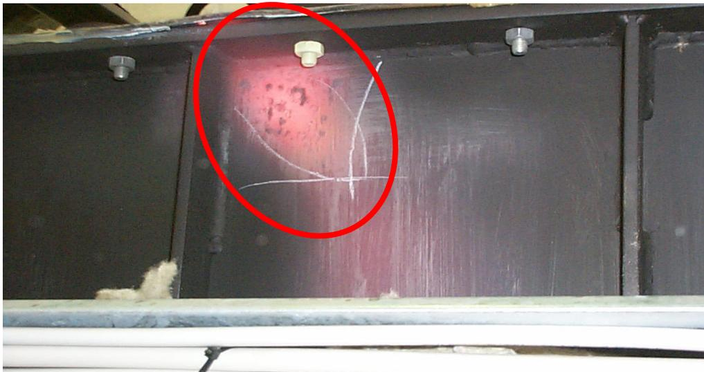
*Figure 3: Consequences of an insulation failure at the gasifier shell.*
