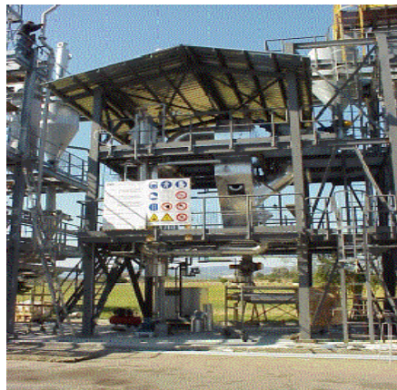
Figure 21: 160 kW e (CFB) Gasification Plant Developed by ENEA and installed in China
