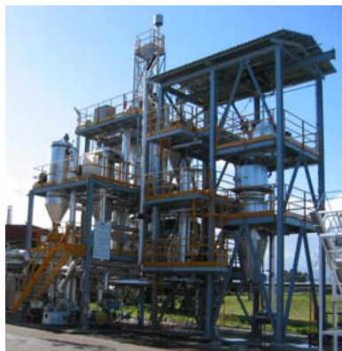
Figure 20: TUV's Fast Internal Circulation Fluidized bed Gasifier at ENEA Trisaia Centre (Capacity: 500 KWth)
