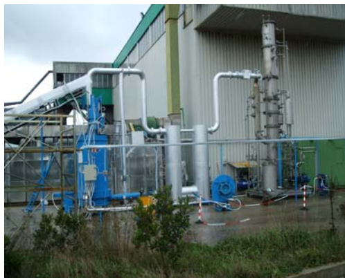
Figure 22: Horizontal Fixed Bed gasifier in Tempio Pausania (Sardinia); capacity 1.5 KWth
