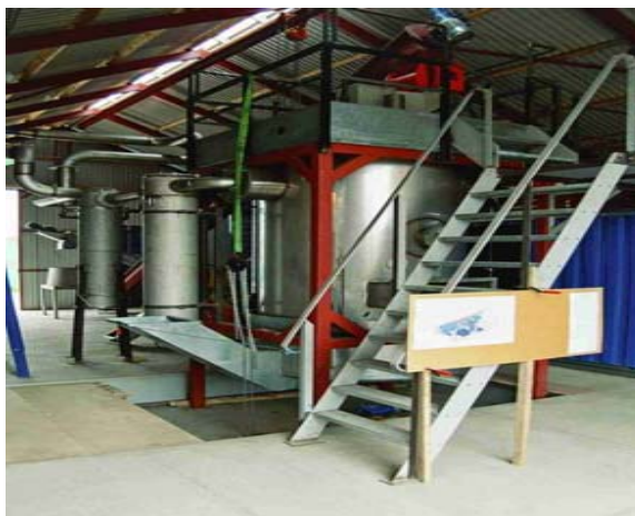
Figure 5: The Castor Gasification CHP Pilot Plant at Græsted (Electricity = 23%, Heat = 53%, Heat Losses = 24%)
