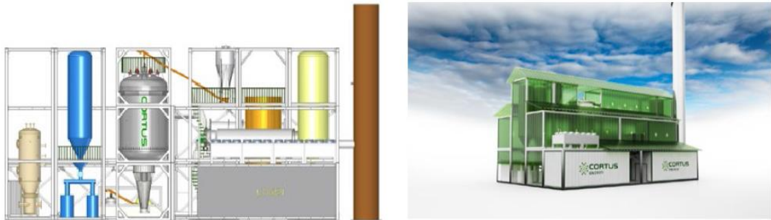
Figure 63: Cortus Wood Roll 6 MW thermal CHP module
