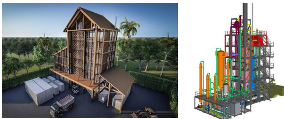
Figure 40: Synova's waste-to-power plant with power block for 1.5 MW e in two different designs
