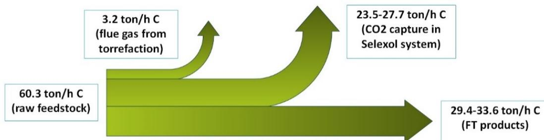
Figure 3. Carbon balance over the FT process and carbon capture efficiency.
