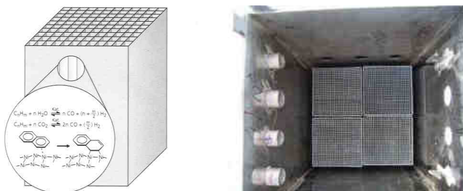
Figure 2-7 Tar reforming monolith and monolith reactor unit
