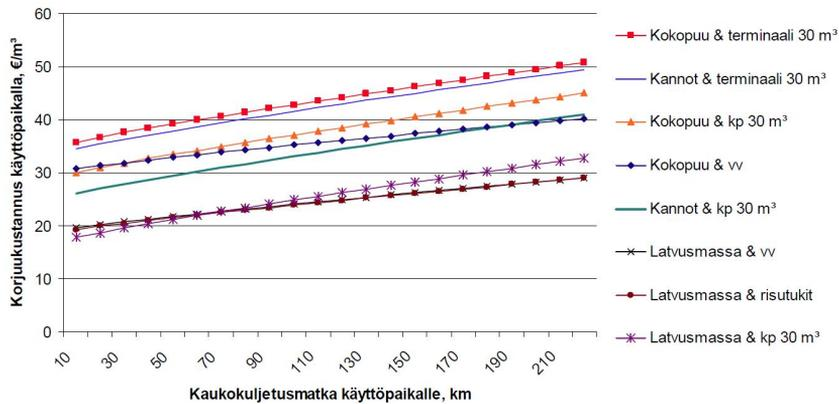
**Figure 17.** Cost of biomass at plant gate as a function of transportation distance for different harvesting techniques and forest biomass types.
