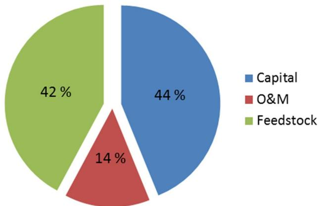
**Figure 33.** Breakdown of annual costs for a typical BTL plant examined in this work using case LTFT-1 as an example.
