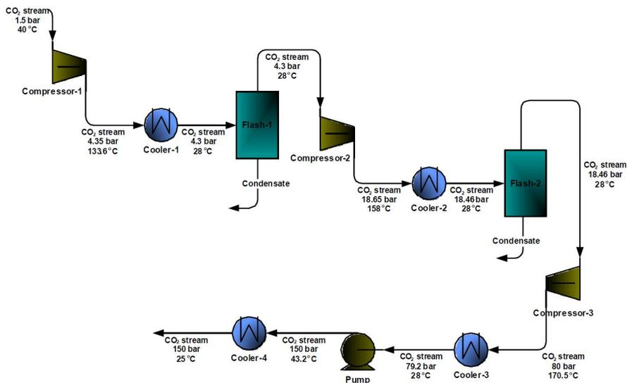
**Figure 14.** Flow diagram of a CO<sub>2</sub> compression step according to the CAESAR guideline.<sup>33</sup>
