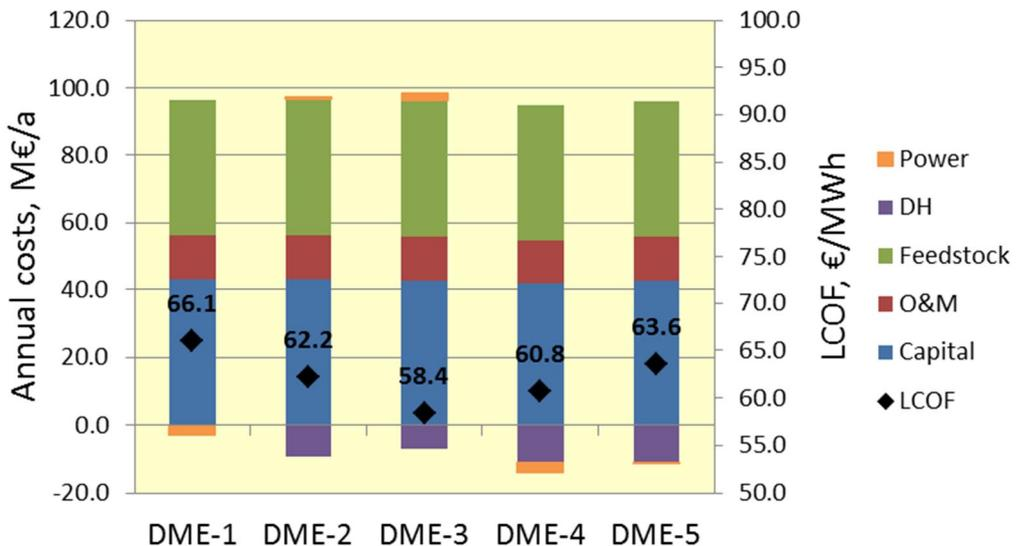
**Figure 22.** Annual cost estimates (columns) and levelised production costs (dots) for the simulated single-step DME plant designs.
