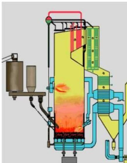
**Figure 11.** An example of a biomass bubbling fluidised-bed boiler by Foster Wheeler.<sup>32</sup>
