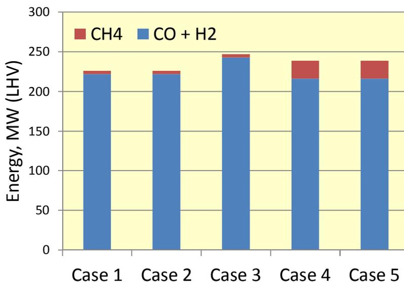
**Figure 15.** Comparison of the cold gas efficiency between presented case designs from biomass (dryer input at 50 wt%) to chemical energy of synthesis gas based on lower heating values.
