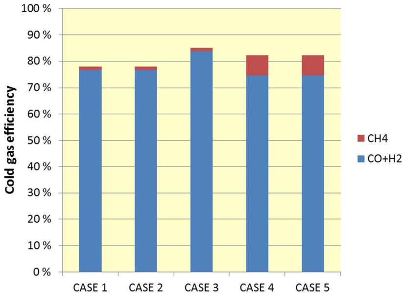
**Figure 38.** Cold gas efficiency (LHV) at the synthesis inlet for each of the cases.
