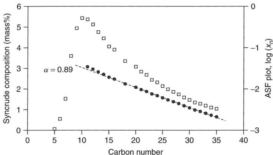
**Figure 23.** Carbon number distribution of the C<sub>5</sub> and heavier products (squares) obtained with the original Co-LTFT catalyst for SMDS, as well as the corresponding ASF-plot (dots).<sup>67</sup>
