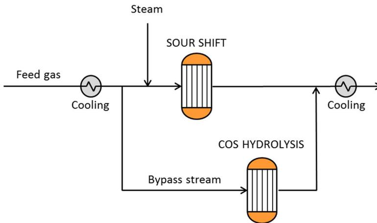
**Figure 8.** Layout of CO shift arrangement.
