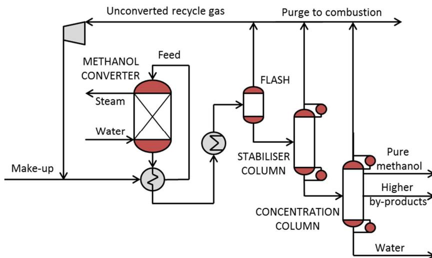
**Figure 19.** Simplified layout of the low-pressure methanol synthesis loop, product recovery and distillation section.
