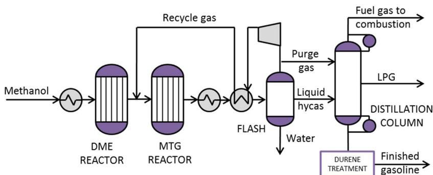
**Figure 26.** Simplified layout of the MTG synthesis, product recovery and distillation section, adapted from [89]. The feed/effluent heat exchangers of the DME and MTG reactors are not shown.
