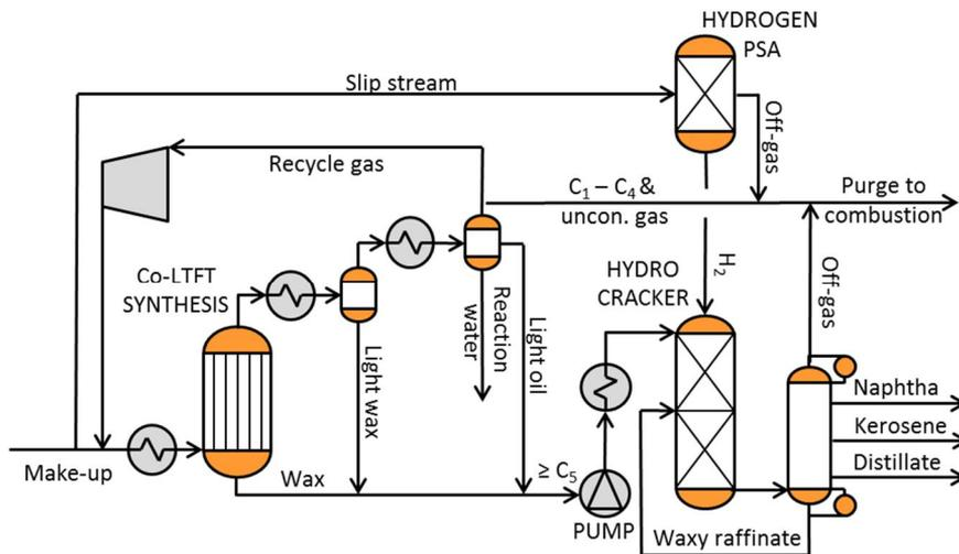
**Figure 24.** Simplified layout of the FT synthesis, product recovery and refinery section, adapted from the SMDS design in Ref. 67. As the upgrading area operates at higher pressure than the FT reactor, the waxes and light oil needs to be pumped prior inlet to the hydrocracker.
