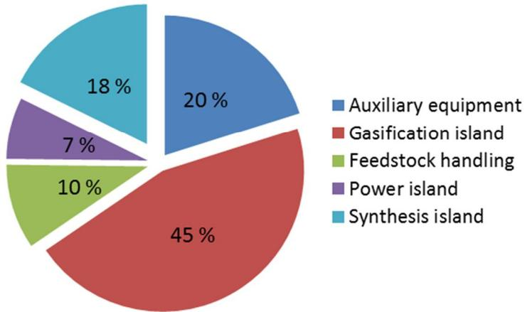
**Figure 32.** Capital breakdown for a typical BTL plant examined in this work using case MEOH-1 as an example.
