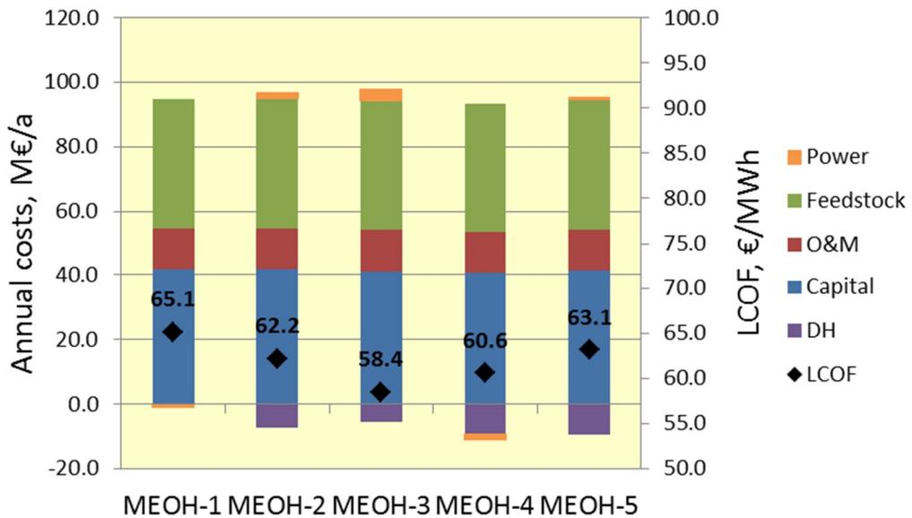
**Figure 20.** Annual cost estimates (columns) and levelised production costs (dots) for the simulated methanol plant designs.
