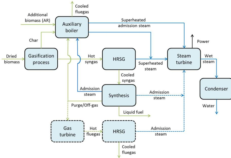
**Figure 12.** A possible layout for a BTL plant's steam system. The final setup is specific to scale, type of synthesis and arrangement of recycle loops.
