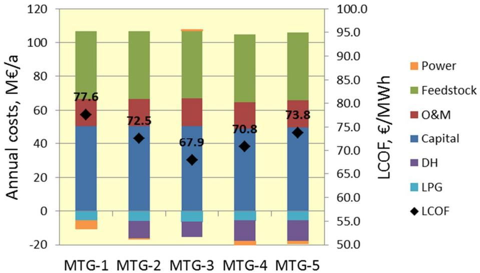
**Figure 27.** Annual cost estimates (columns) and levelised production costs (dots) for the simulated MTG plant designs.
