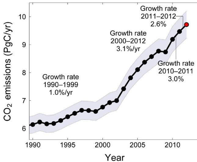
**Figure 1.** Global CO<sub>2</sub> emissions from fossil fuel combustion and cement production including an uncertainty of  $\pm 5\%$  (grey shading). Emissions projection for year 2012 is based on GDP projection (red dot).<sup>6</sup>
