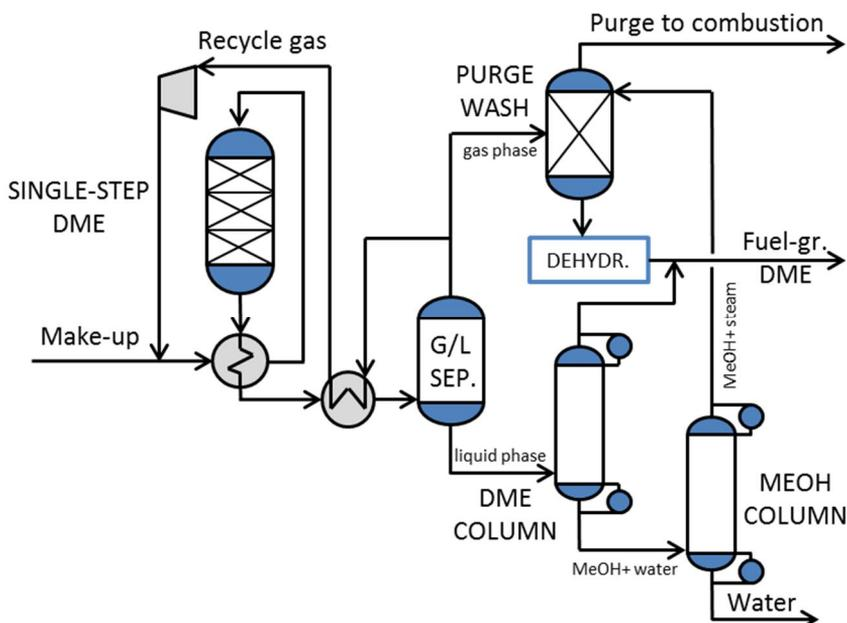
**Figure 21.** Simplified layout of the single-step DME synthesis, product recovery and distillation section, adapted from [55] and [56]. The reactor features three layers of mixed methanol and dehydrations catalysts with intercooling (not shown).
