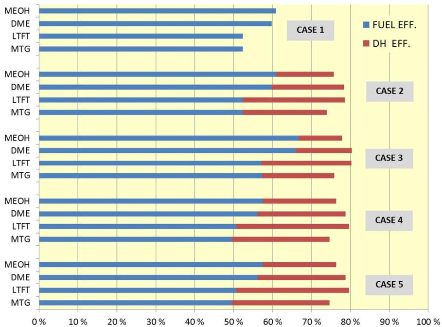
**Figure 29.** Overall efficiencies from biomass to fuel and byproduct district heat for the selected plant designs. The MTG fuel efficiency column excludes LPG.
