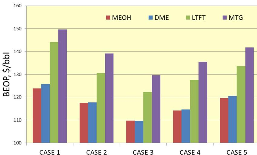
**Figure 37.** Calculated breakeven oil prices (BEOP) for the selected plant designs using 0.3 \$/gal refining margin. Long-term crude oil price forecasts by IEA & EIA are in the range of 108–134 \$/bbl (in 2010 dollars).
