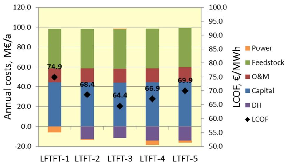
**Figure 25.** Annual cost estimates (columns) and levelised production costs (dots) for the simulated FT plant designs.
