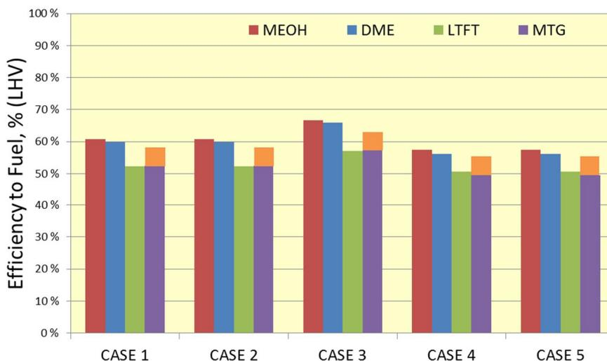
**Figure 28.** Summary of overall efficiencies from biomass to fuel for the selected plant designs. The orange rectangle stacked above the MTG column illustrates the amount of byproduct LPG.
