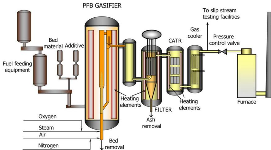
**Figure 6.** VTT's test-rig for the Ultra-Clean Gas process.<sup>17</sup>
