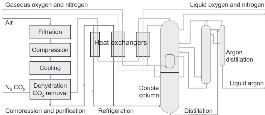
**Figure 10.** Flow scheme of a cryogenic air separation unit.<sup>31</sup>
