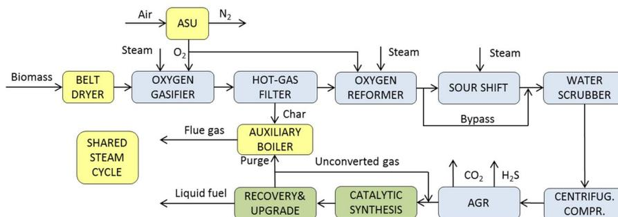
**Figure 5.** Generalised block diagram of a stand-alone biomass-to-liquids plant examined in this work.
