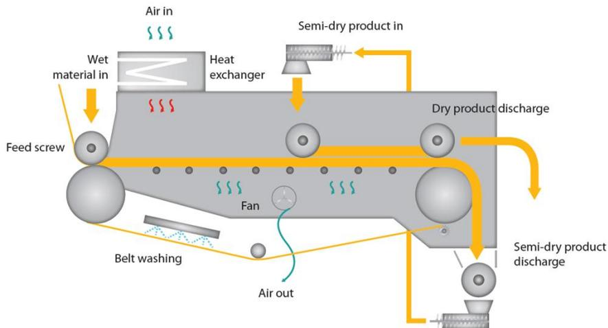
**Figure 9.** A schematic of a KUVO belt dryer.<sup>28</sup>
