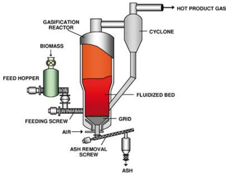
**Figure 7.** A schematic of a bubbling fluidised-bed gasifier for biomass developed and offered by ANDRITZ Carbona.<sup>20</sup>
