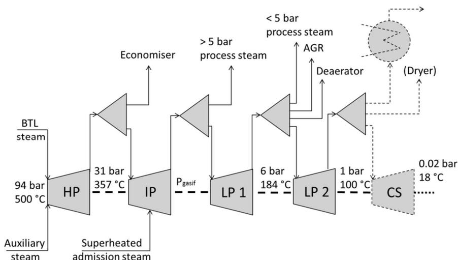
**Figure 13.** Block diagram illustrating our extraction steam turbine design.
