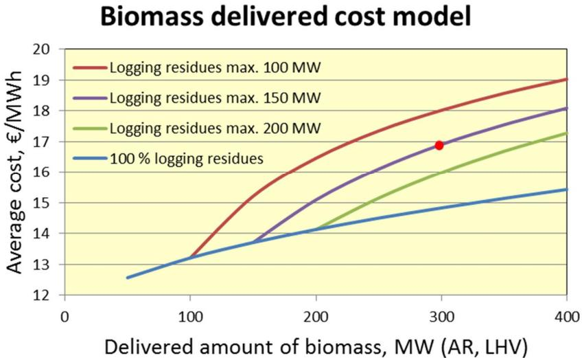
**Figure 18.** Cost curves for biomass feedstock as a function of transportation distance with different maximum amounts of logging residues assuming costs and availabilities discussed in the text.
