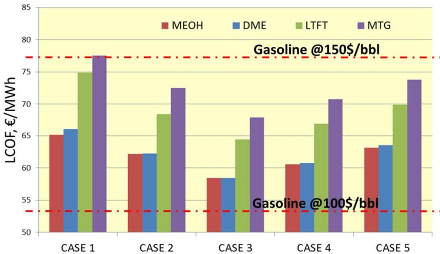
**Figure 31.** Summary of levelised production cost estimates of fuel (LCOF) for the examined plant designs. The horizontal red lines show the comparable price of gasoline (before tax, refining margin 0.3 \$/gal, exchange rate: 1 € = 1.326 \$) with crude oil prices 100 \$/bbl and 150 \$/bbl. The cost estimates have been calculated for mature technology at 300 MWth (of biomass) scale, without investment support, CO<sub>2</sub> credits or tax assumptions.
