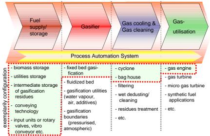
Figure 2-1: Typical process chain of a biomass cogeneration plant (compare [1])
