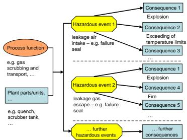
Figure 4-3 Structure of hazard identification
