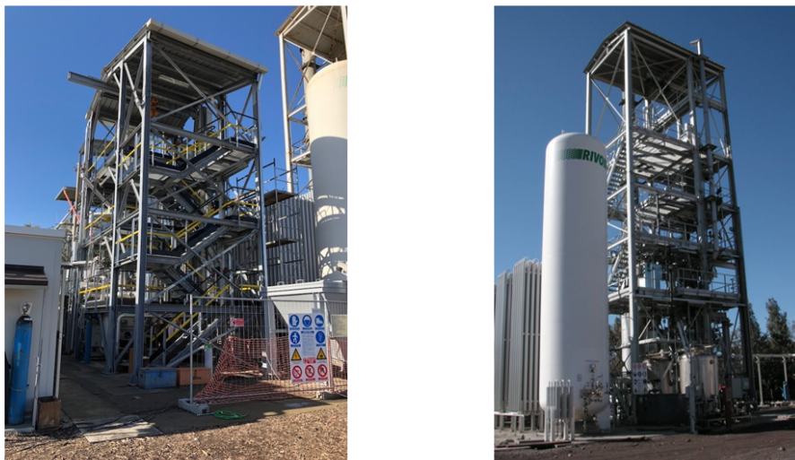
Figure 6: Pilot scale bubbling fluidized bed unit (500 kWth) - left side, demo-scale fixed bed gasification unit (5 MWth) - right side
