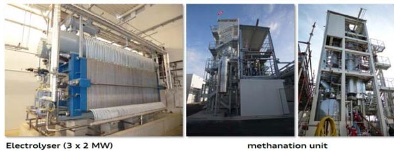
Figure 38: Electrolyser and methanation units (source: Audi)
