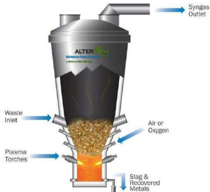
Figure 64 The AlterNRG plasma gasifier 328 .
