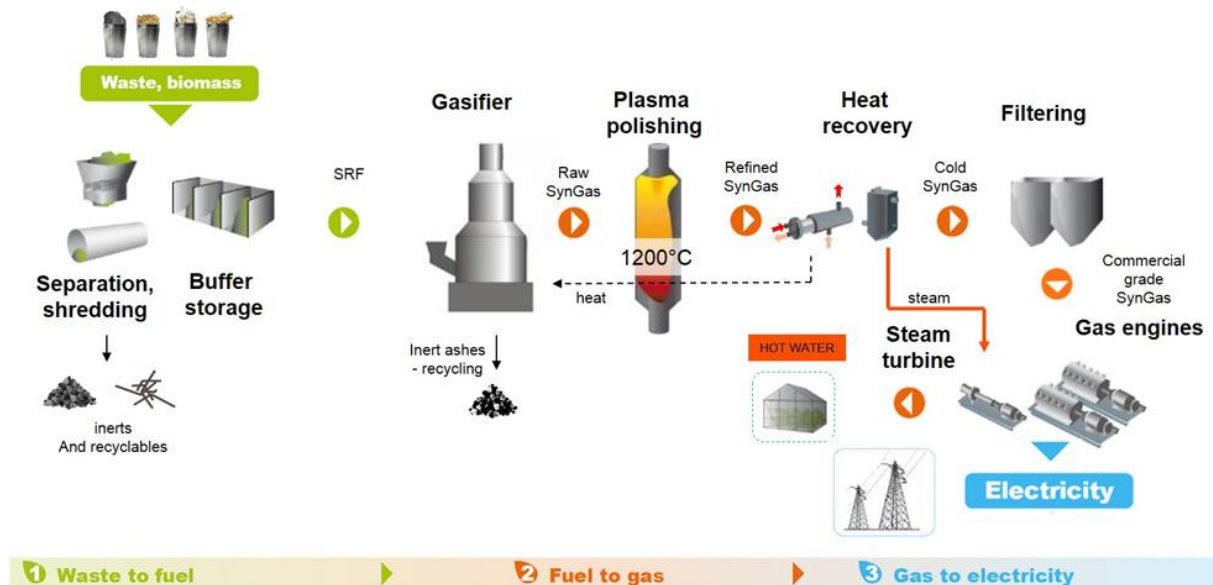
Figure 65 Process flow schematic for the CHO Power process 333 .
